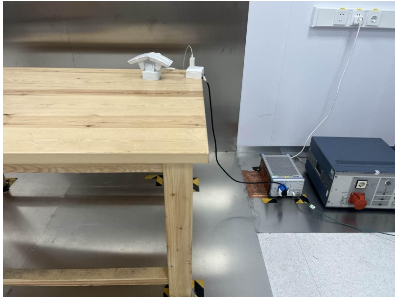
Radiated Emission Test View|(Below 1G)
