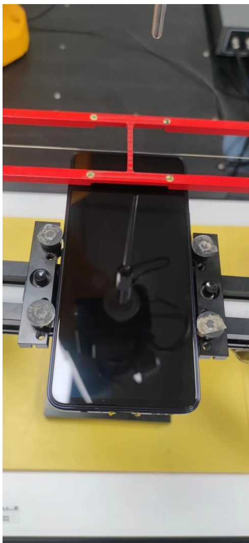
Picture 2: EUT Positioning for RF/T-coil
