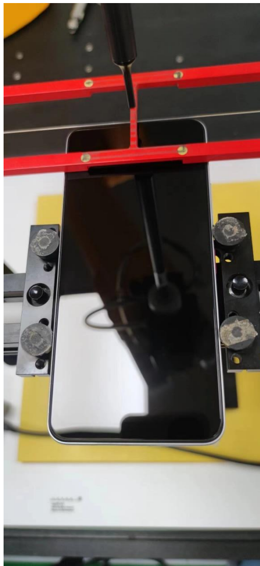
Picture 2: EUT Positioning for RF/T-coil
