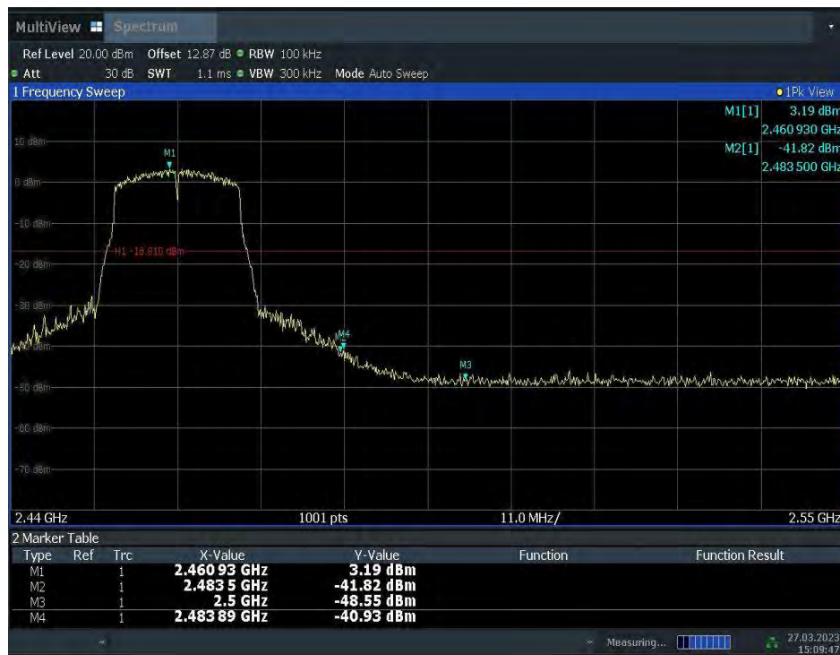
Fig.A.5.4 Band Edges (802.11g, Ch 11)
