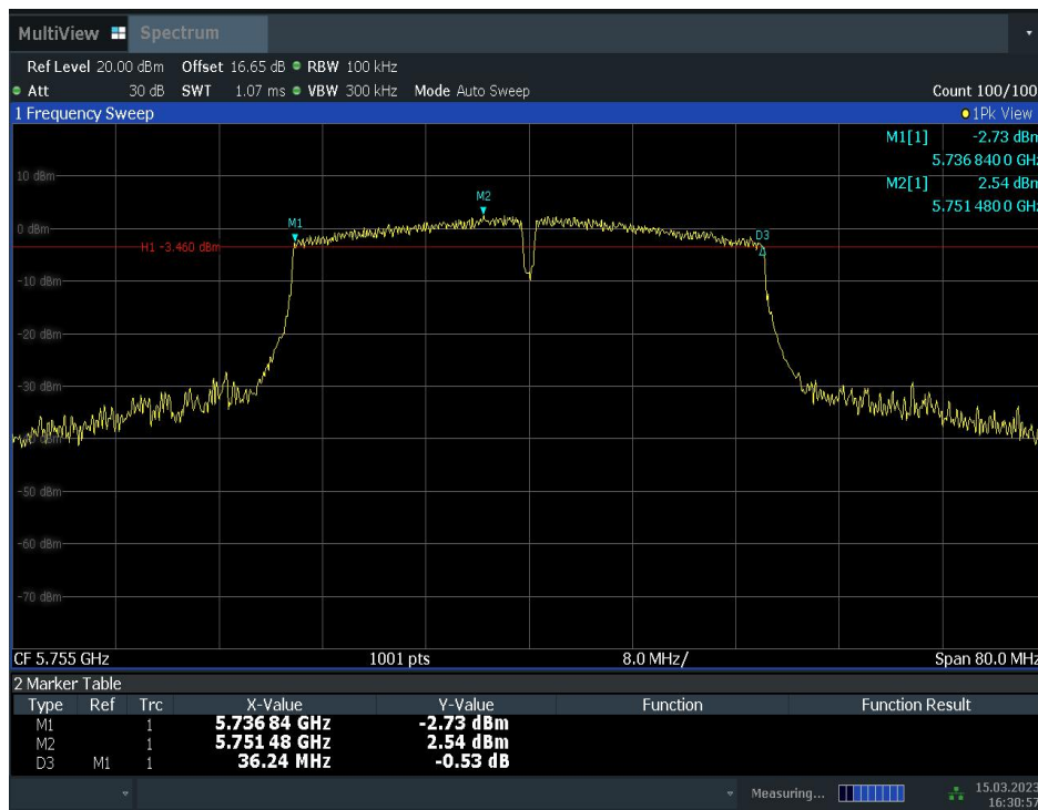
Fig. 7 Occupied 6dB Bandwidth (802.11n-HT40, Ch 151)
