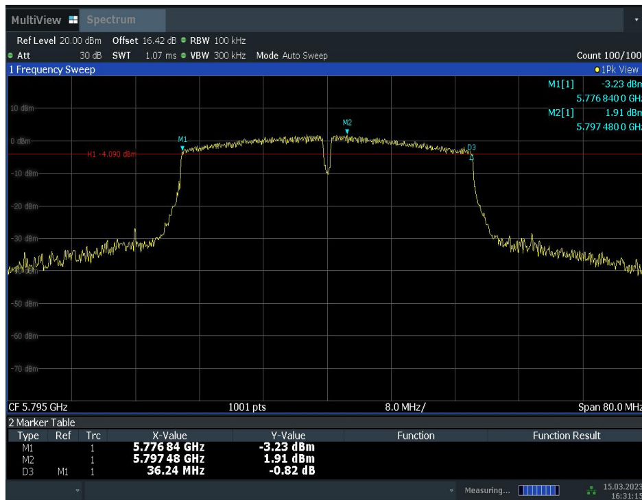
Fig. 7 Occupied 6dB Bandwidth (802.11n-HT40, Ch 151)
