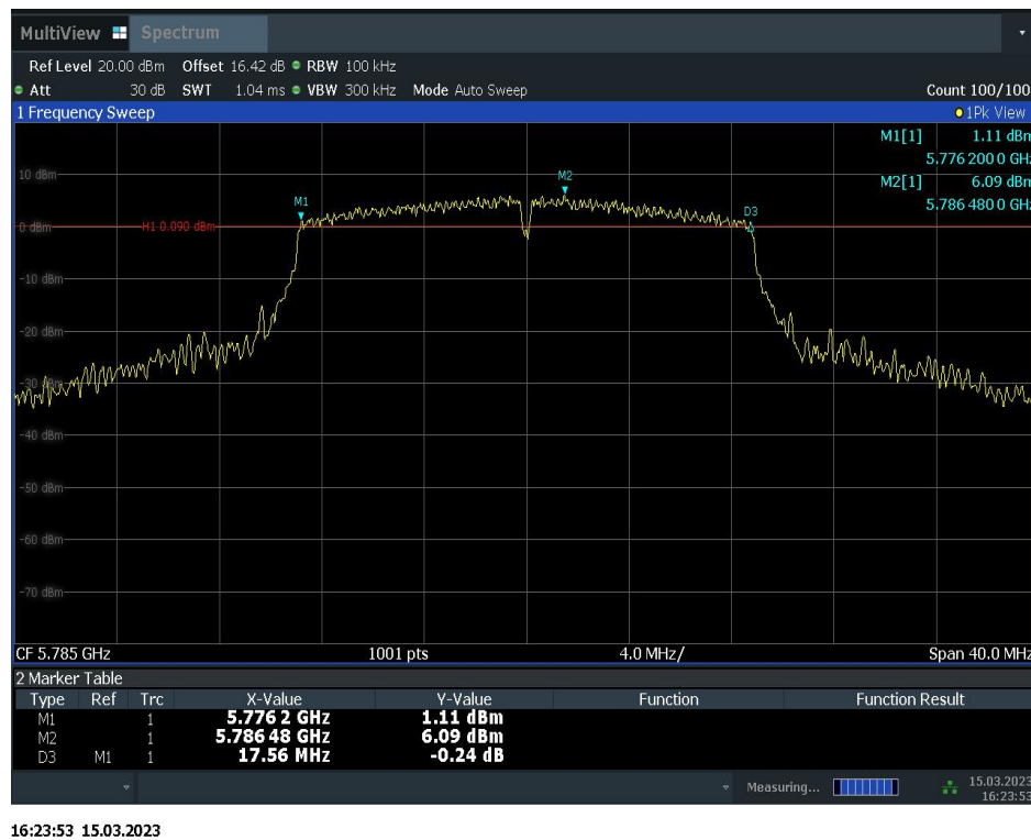
Fig. 5 Occupied 6dB Bandwidth (802.11n-HT20, Ch 157)
