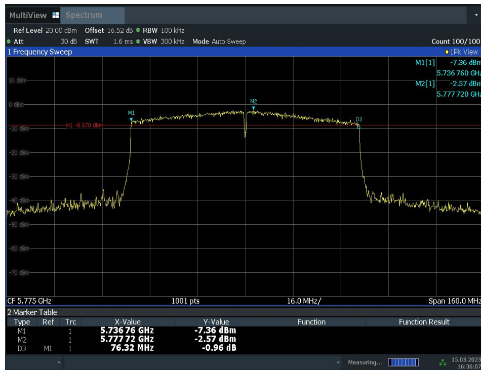
Fig. 9 Occupied 6dB Bandwidth (802.11ac-HT80, Ch 155)
