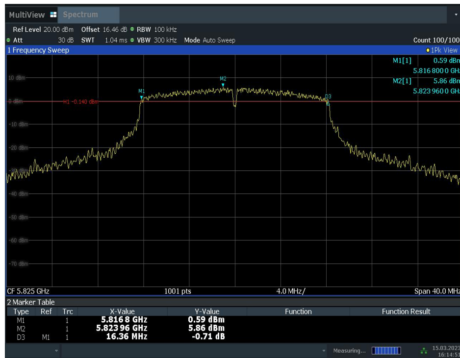
Fig. 3 Occupied 6dB Bandwidth (802.11a, Ch 165)
