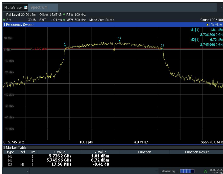
Fig. 4 Occupied 6dB Bandwidth (802.11n-HT20, Ch 149)
