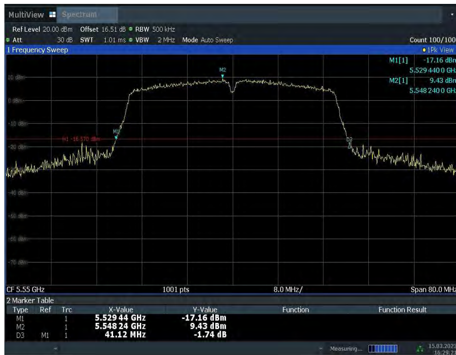
Fig.26 Occupied 26dB Bandwidth (802. 11n-HT40, 5590MHz)
