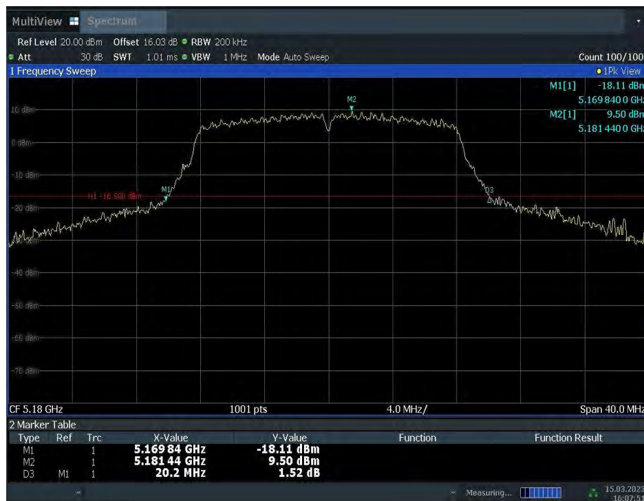
Fig.1 Occupied 26dB Bandwidth (802.11a, 5180MHz)
