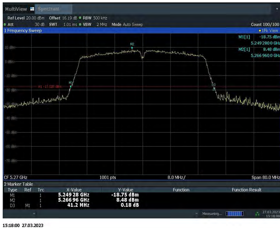
Fig.23 Occupied 26dB Bandwidth (802.11n-HT40, 5270MHz)
