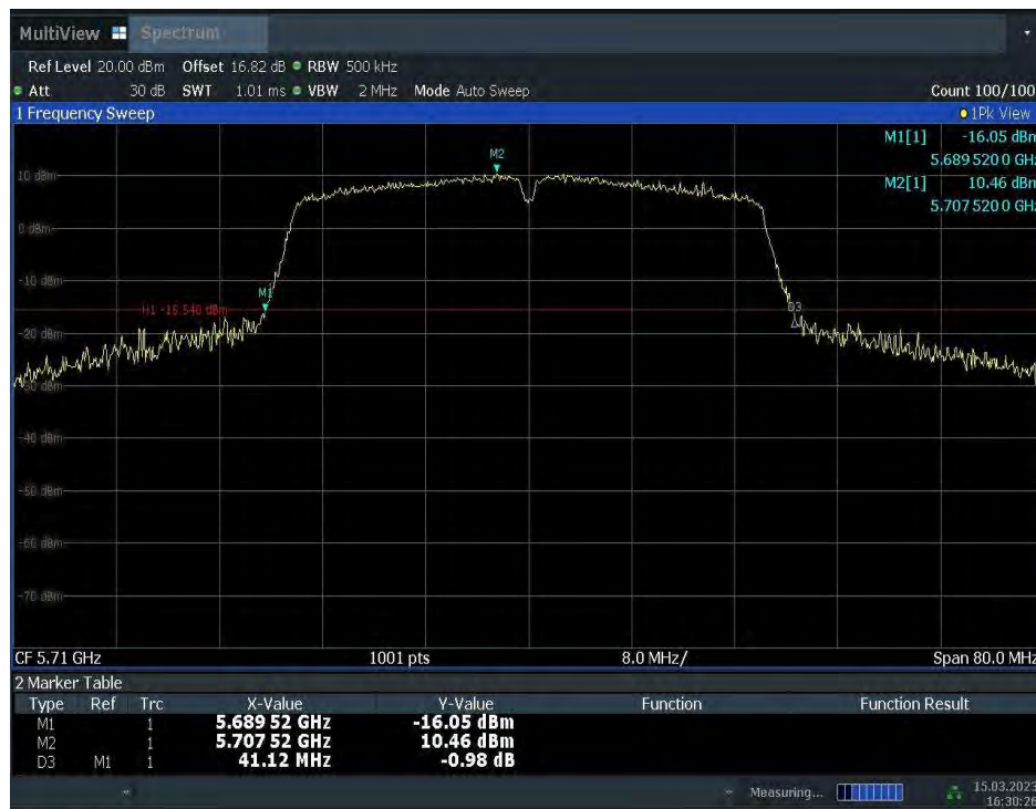
Fig.28 Occupied 26dB Bandwidth (802. 11n-HT40, 5710MHz)
