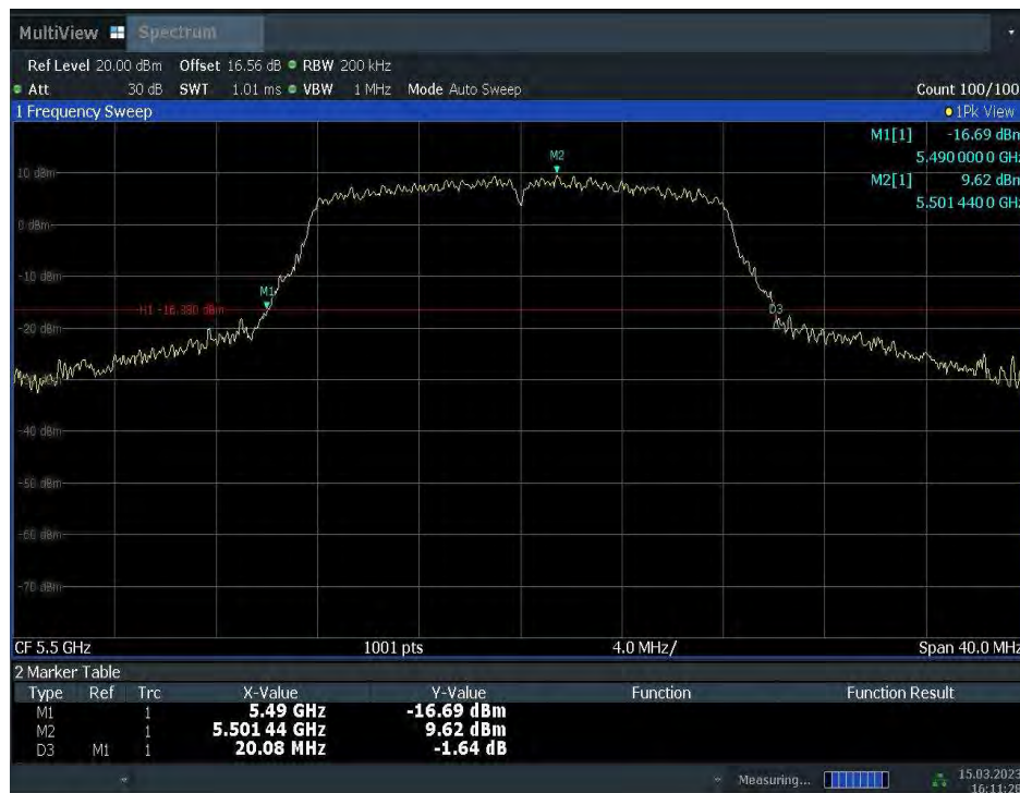
Fig.7 Occupied 26dB Bandwidth (802.11a, 5500MHz)
