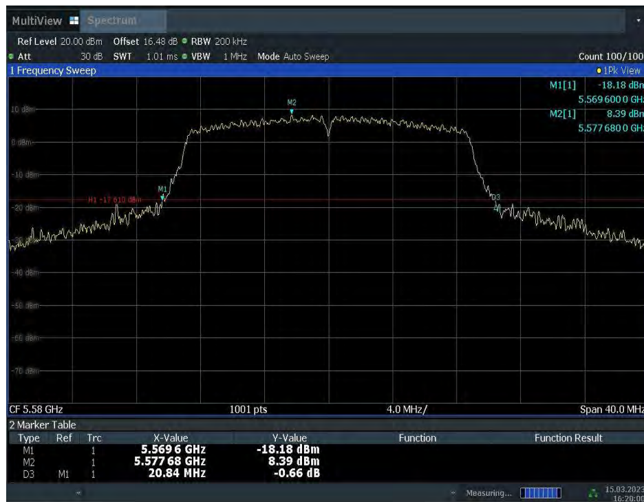
Fig.18 Occupied 26dB Bandwidth (802. 11n-HT20, 5580MHz)
