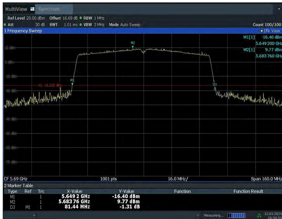
Fig.33 Occupied 26dB Bandwidth (802. 11ac-HT80, 5690MHz)
