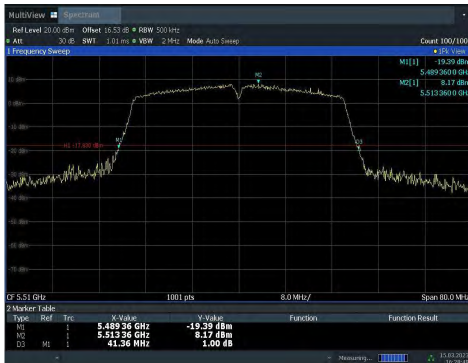
Fig.25 Occupied 26dB Bandwidth (802.11n-HT40, 5510MHz)
