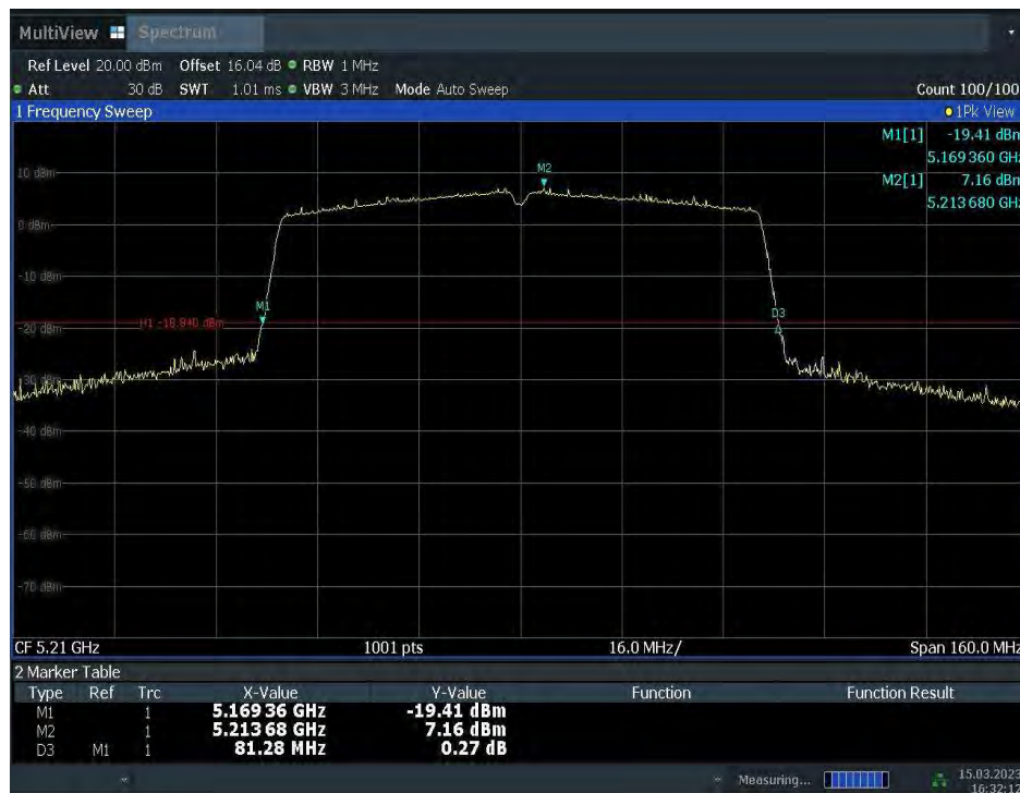
Fig.29 Occupied 26dB Bandwidth (802. 11ac-HT80, 5210MHz)
