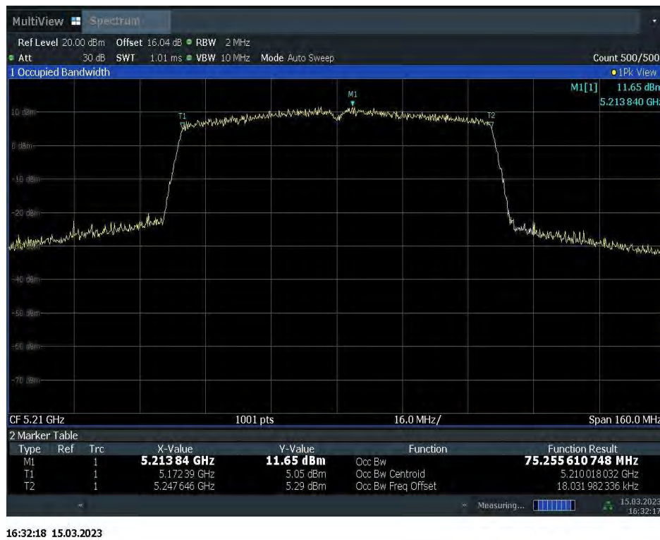
Fig.68 99% Occupied bandwidth (802.11ac-HT80, 5210MHz)
