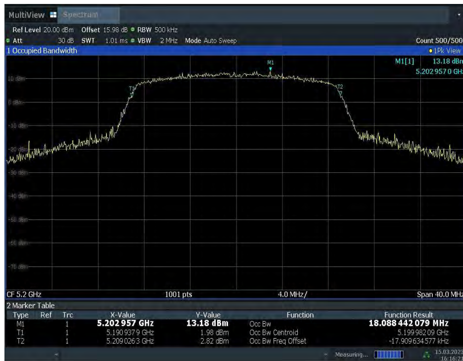
Fig.64 99% Occupied bandwidth (802.11n-HT20, 5200MHz)
