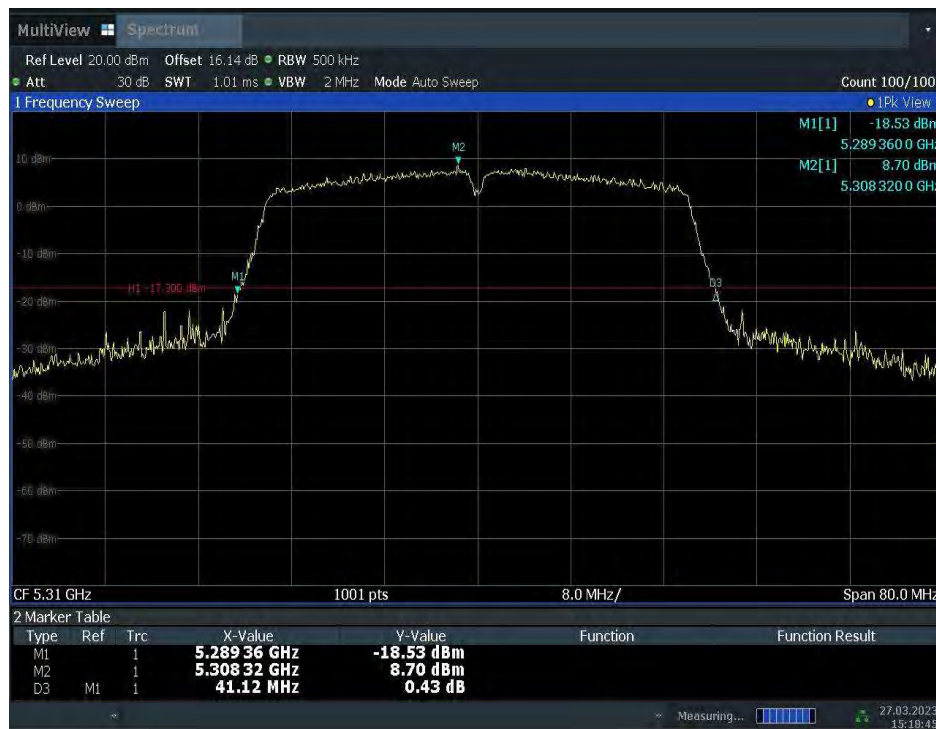
Fig.24 Occupied 26dB Bandwidth (802.11n-HT40, 5310MHz)
