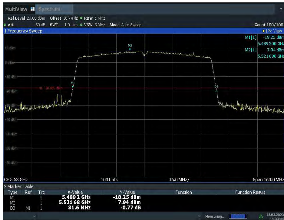
Fig.31 Occupied 26dB Bandwidth (802. 11ac-HT80, 5530MHz)
