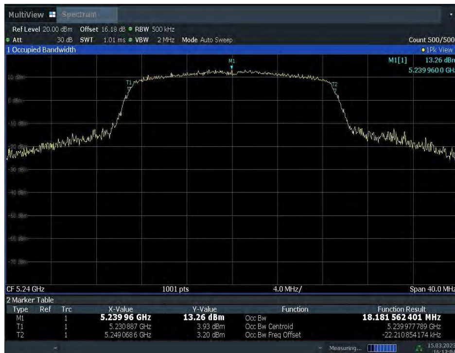
Fig.65 99% Occupied bandwidth (802.11n-HT20, 5240MHz)
