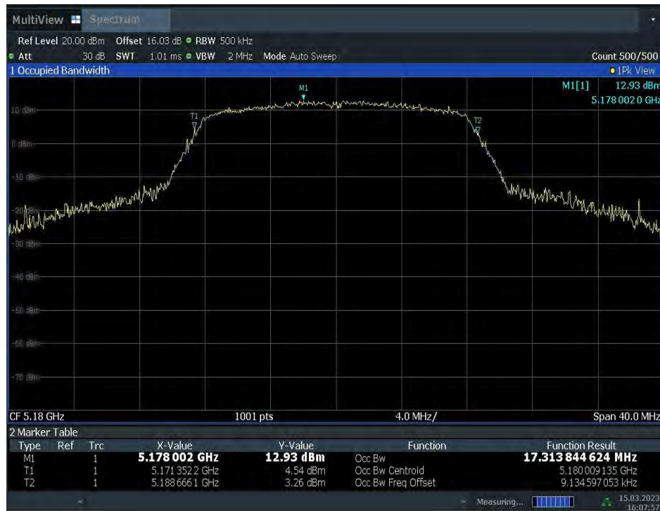
Fig.60 99% Occupied bandwidth (802.11a, 5180MHz)
