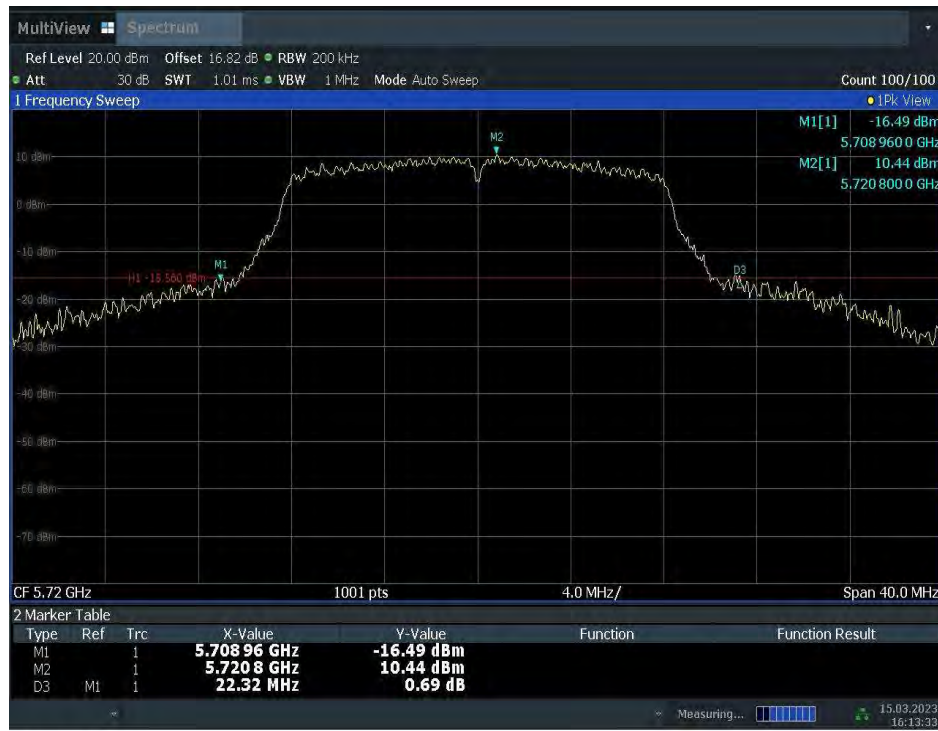
Fig.10 Occupied 26dB Bandwidth (802.11a, 5720MHz)
