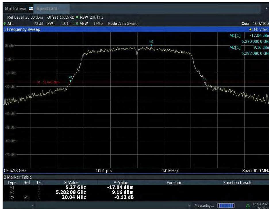
Fig.5 Occupied 26dB Bandwidth (802.11a, 5280MHz)
