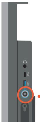
To charge your Grid Pad, plug the Power Supply Unit (PSU) into the charging port on the side of the device. When the Grid Pad is charging the charging indicator is **illuminated white**.
