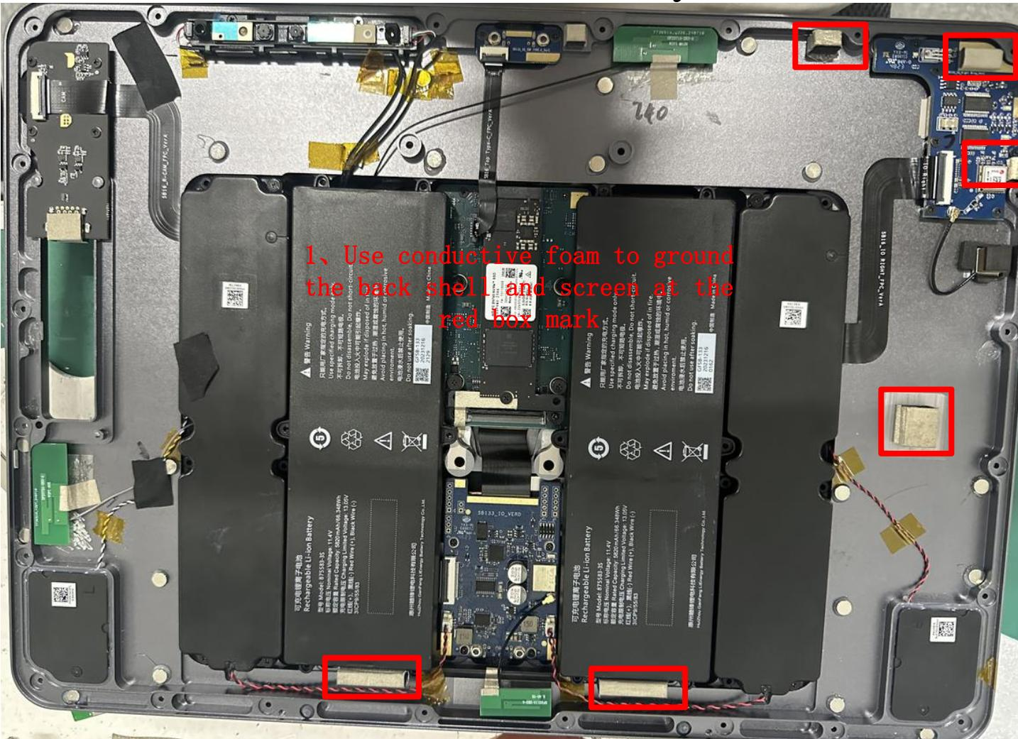
1、Use conductive foam to ground the back shell and screen at the red box mark
