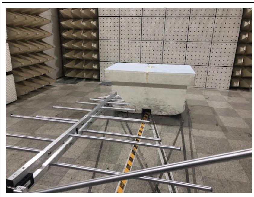
**3. Photo of Radiated Spurious Emission Test (Above 1 GHz)**
