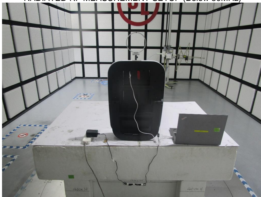
RADIATED RF MEASUREMENT SETUP (Below 30MHz)
