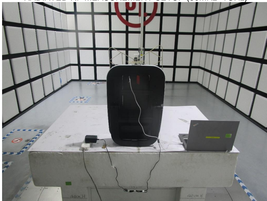
RADIATED RF MEASUREMENT SETUP (Below 30MHz)
