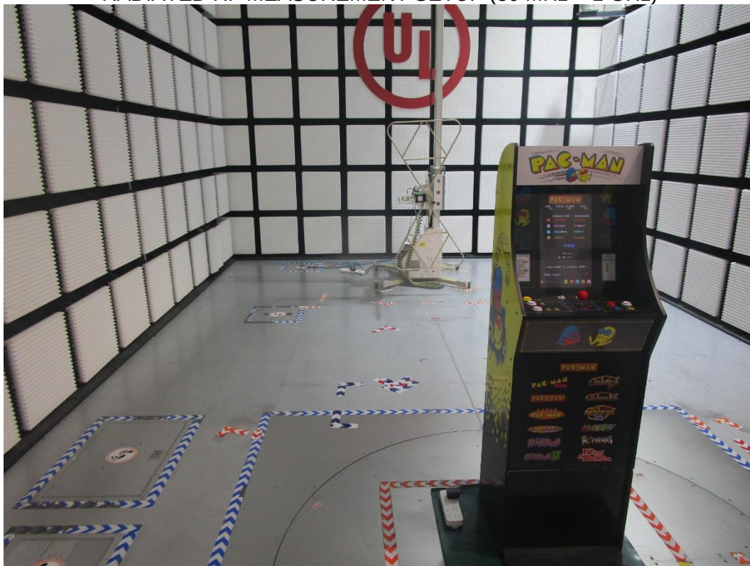
RADIATED RF MEASUREMENT SETUP (Below 30 MHz)
