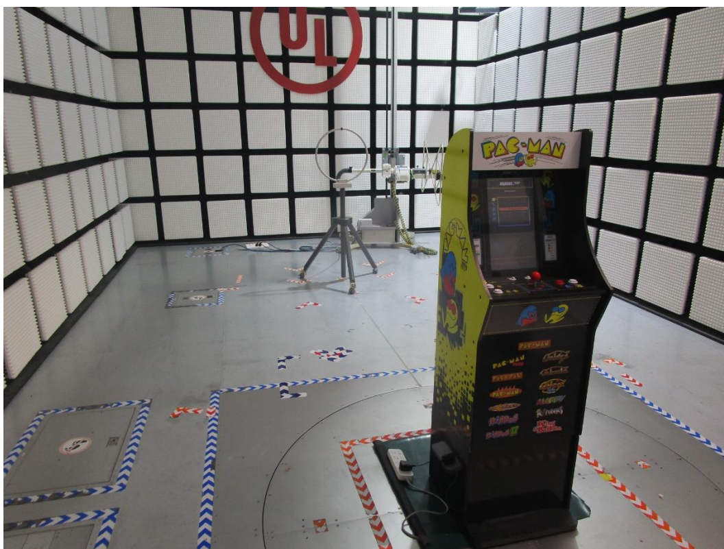
RADIATED RF MEASUREMENT SETUP (Below 30 MHz)
