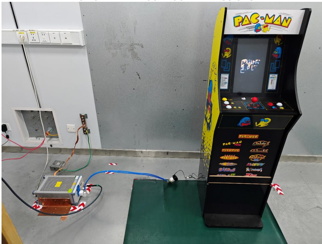
AC POWER LINE CONDUCTED EMISSIONS
