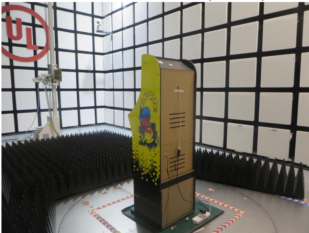
RADIATED RF MEASUREMENT SETUP (Above 1 GHz)
