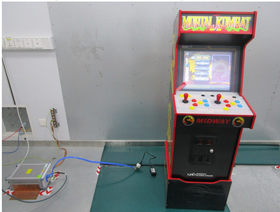
Conducted Emission Test for AC Power Port
