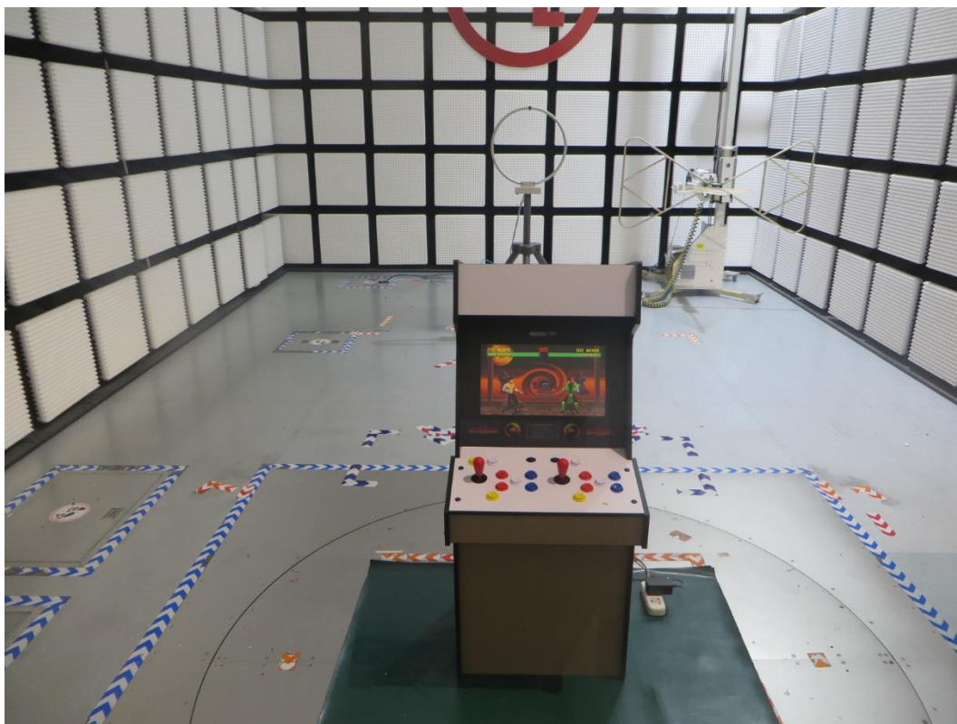
RADIATED RF MEASUREMENT SETUP (Below 30 MHz)
