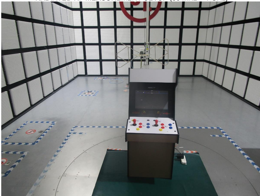
RADIATED RF MEASUREMENT SETUP (Below 30 MHz)
