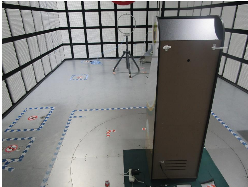
RADIATED RF MEASUREMENT SETUP (Below 30 MHz)
