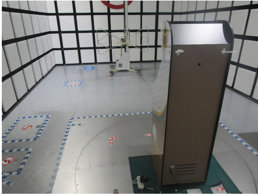
RADIATED RF MEASUREMENT SETUP (30 MHz ~ 1 GHz)
