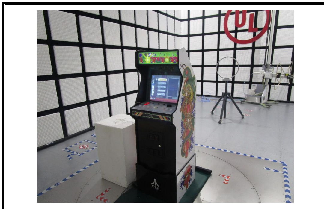
RADIATED RF MEASUREMENT SETUP (Below 30 MHz)
