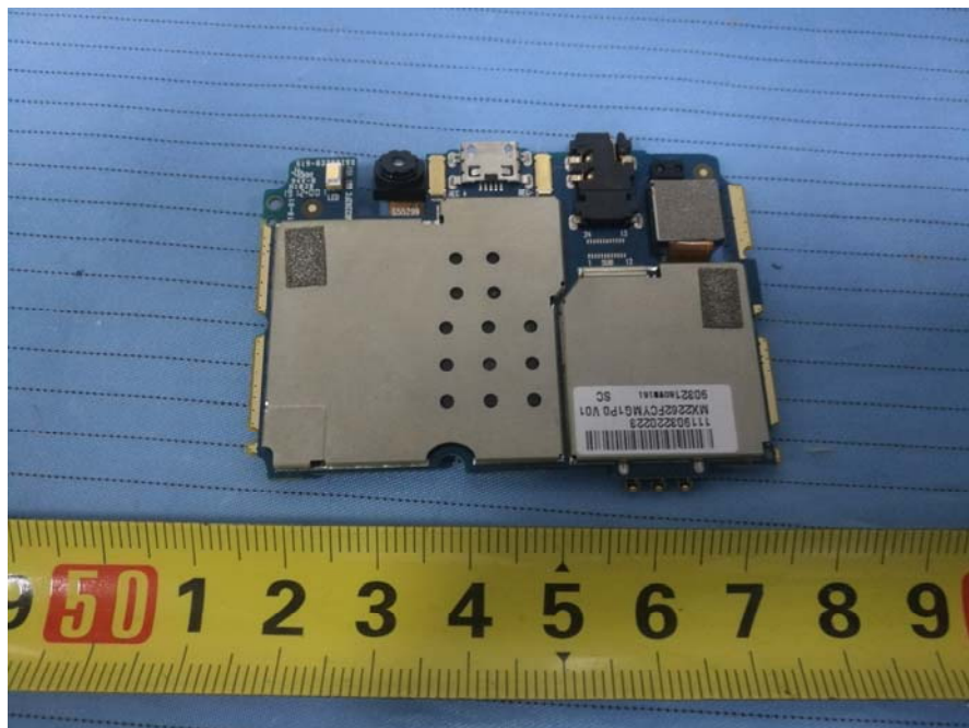
EUT – Mainboard Top View
