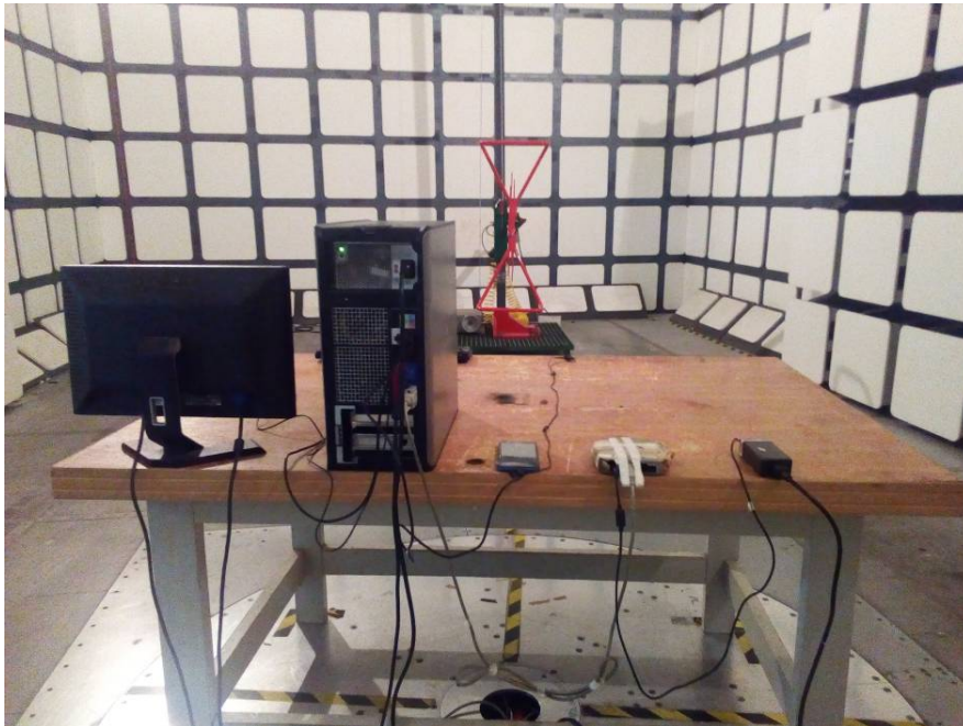
Radiated Emissions – Rear View (Below 1 GHz)
