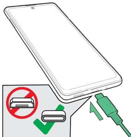
**EN** Insert USB cable and charge for 8 hours
