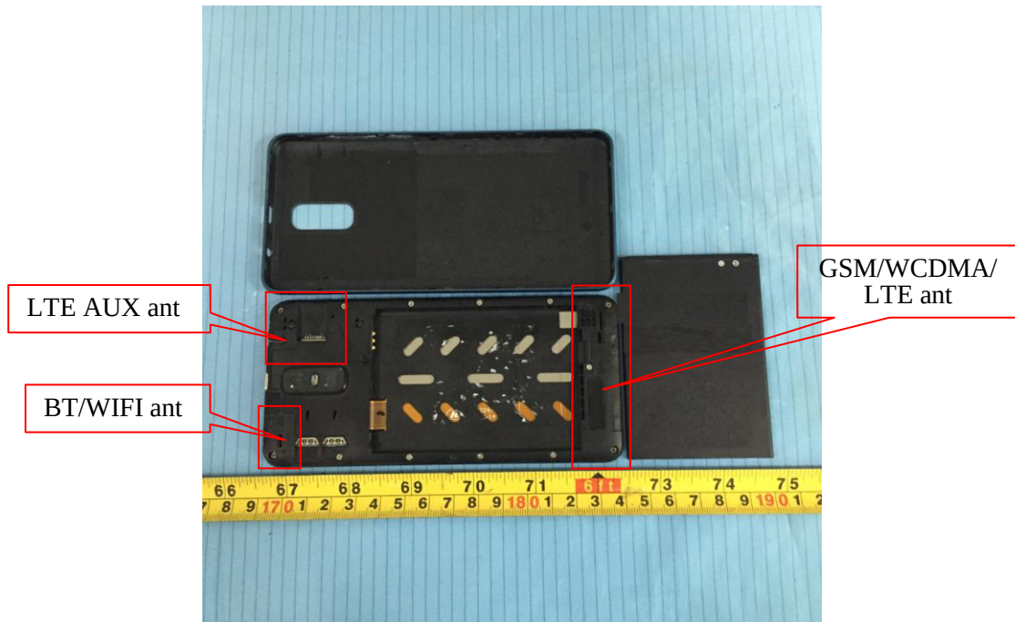
EUT – Cover off View 1
