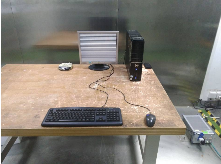
Conducted Emissions - Front View
