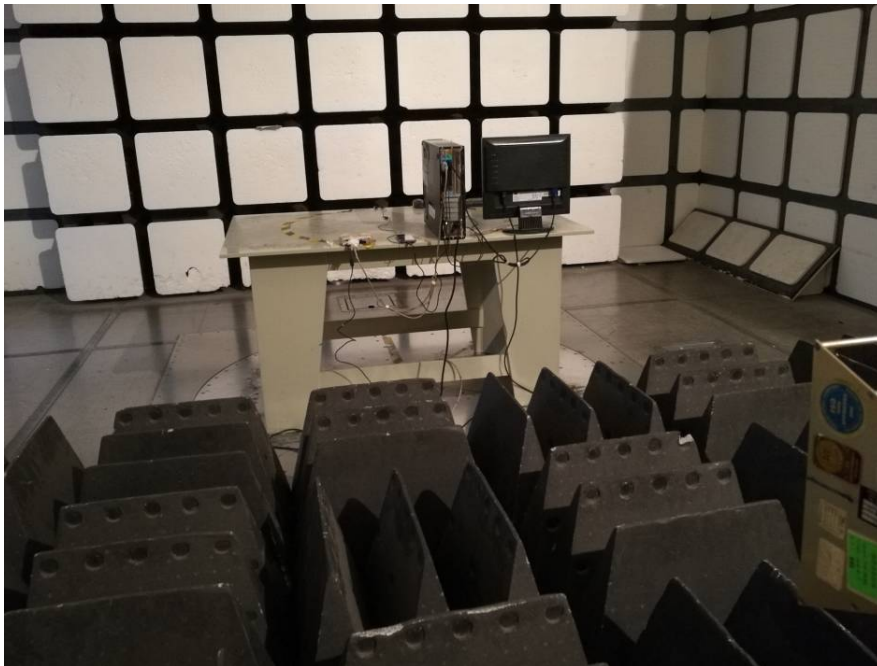
Radiated Emissions – Rear View (Above 1 GHz)
