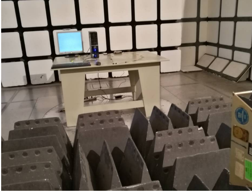
Radiated Emissions – Front View (Above 1 GHz)
