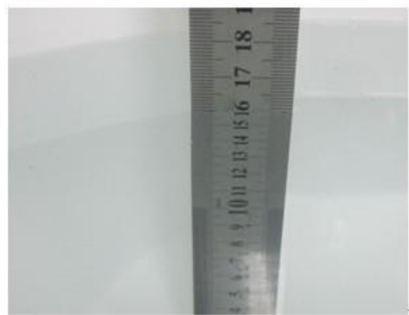
Liquid Height for Body SAR
