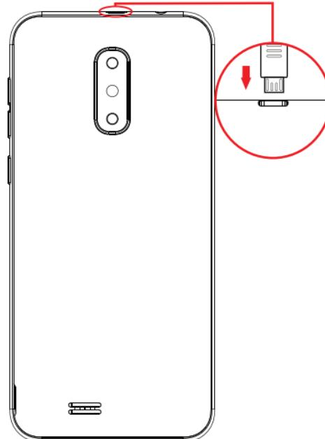
**EN** Insert USB cable and charge for 8 hours
