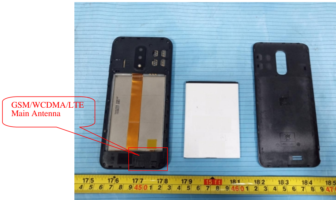
EUT – Cover off View 1
