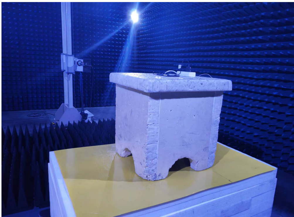
Photo of Radiated Emission Measurement (Above 1G)
