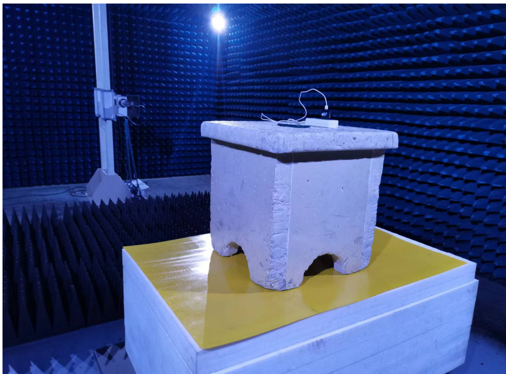
Photo of Radiated Emission Measurement (Above 1G)
