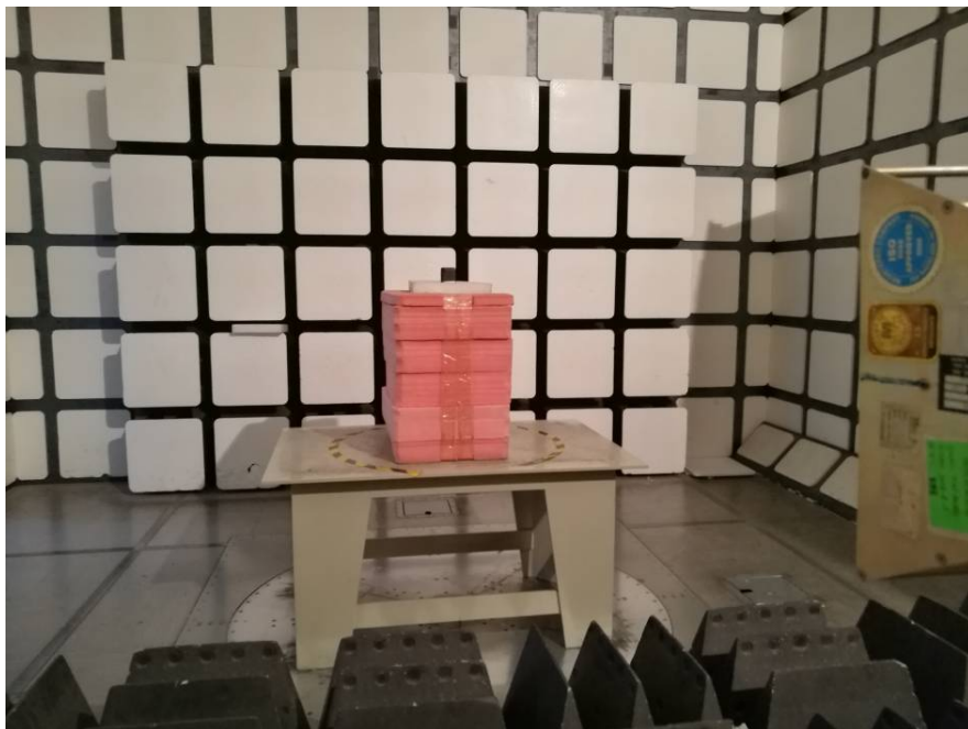
Radiated Emissions View (Above 1 GHz)
