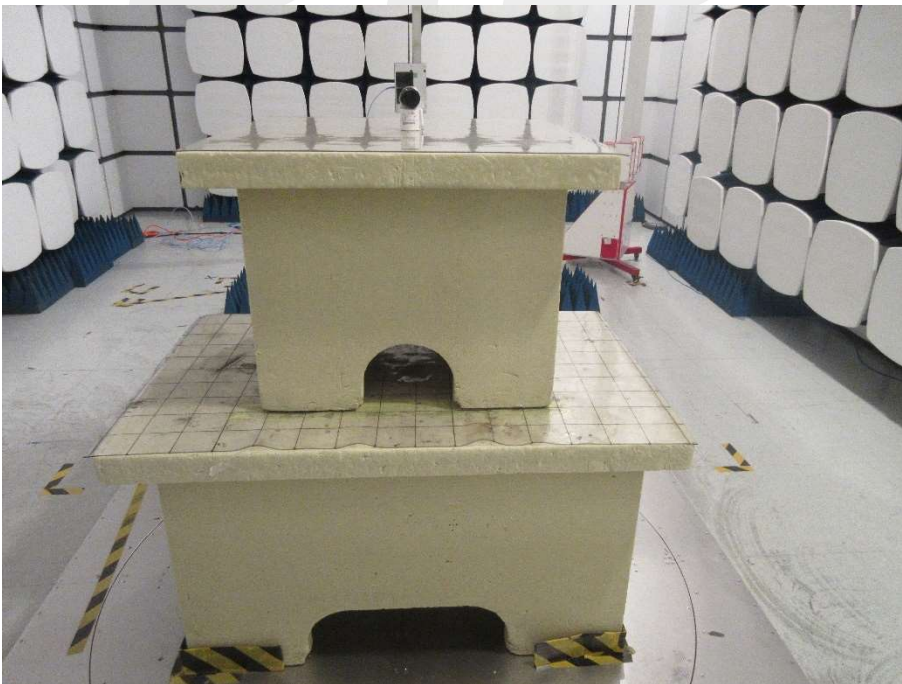
Radiated SPURIOUS EMISSION SET-UP PHOTOS, 1GHz ~ 18GHz
