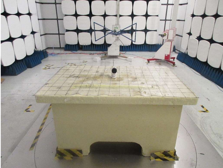
Radiated SPURIOUS EMISSION SET-UP PHOTOS, 30MHz ~ 1GHz
