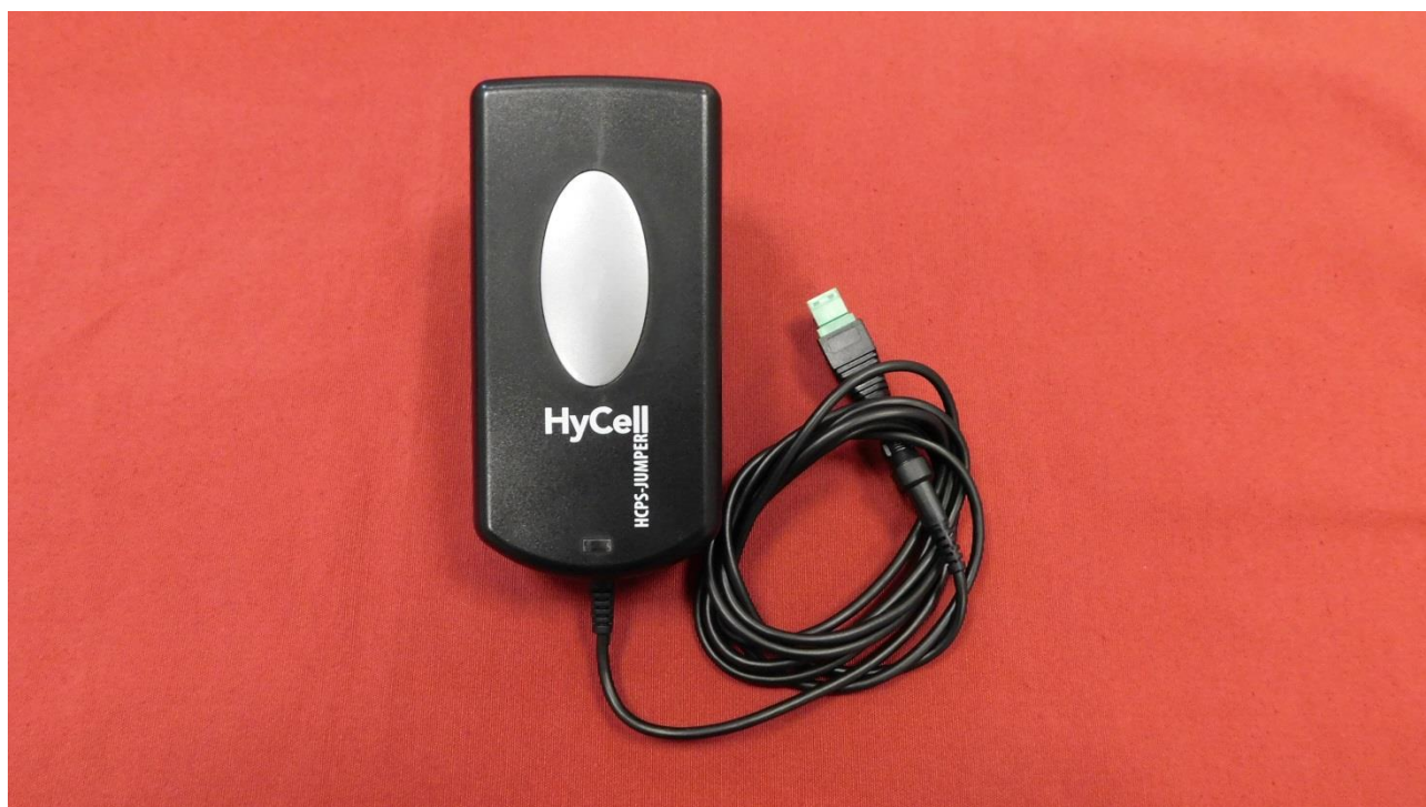
Picture 15: Power supply (only used for AC powerline conducted emissions)
