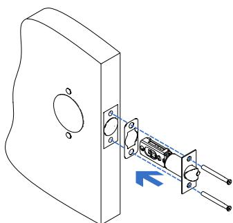
Slide latch into edge bore of the door. Check that the faceplate does not project outside door, but it should also not be installed sunk.
