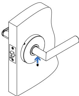
Insert the locking screw from the bottom of the mechanical door handle and tighten it.
