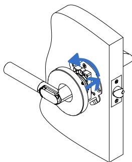
Attach the covers of both the door handles by placing it on the holder and turning it.
