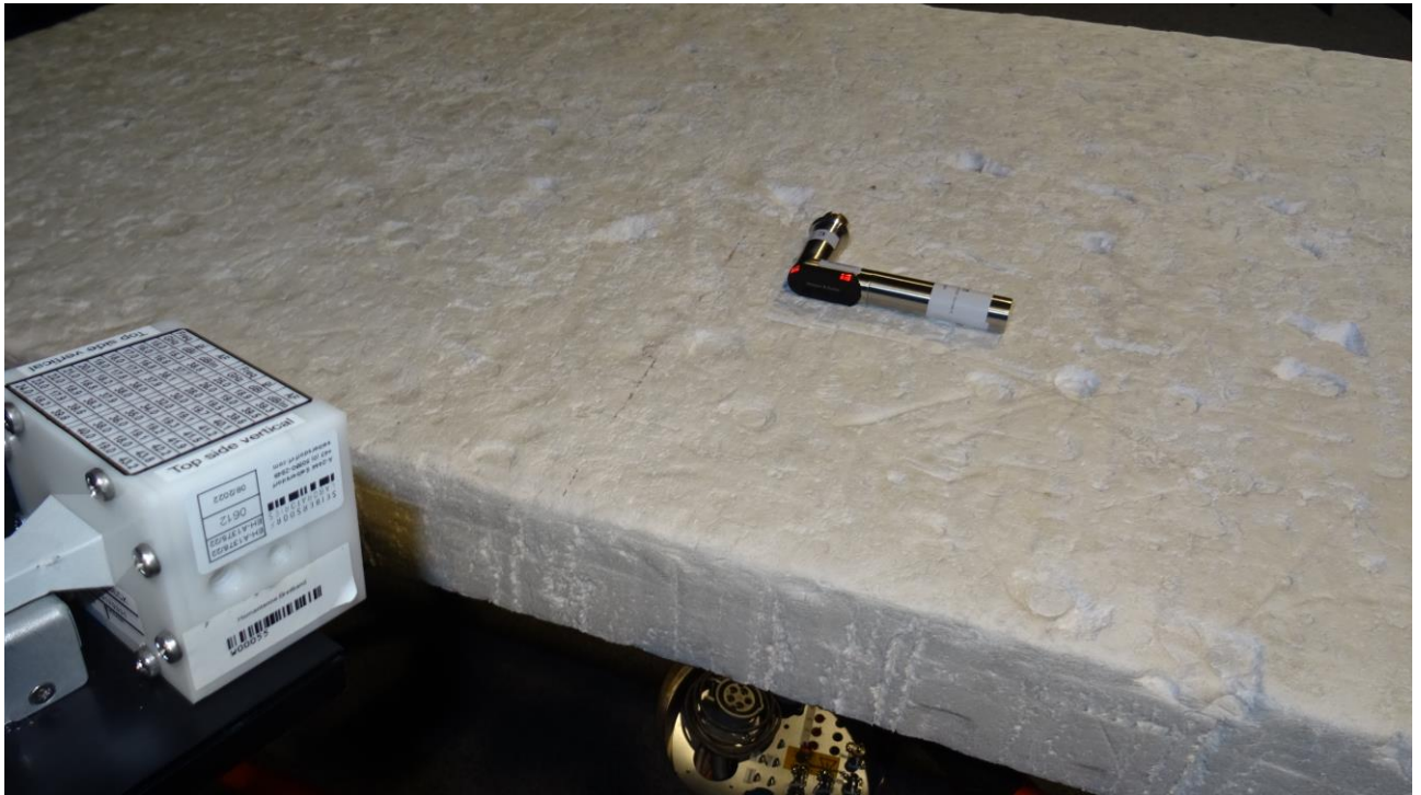
Picture 7: FS-SAC, exploratory radiated emission test 17 GHz – 25 GHz (front view)
