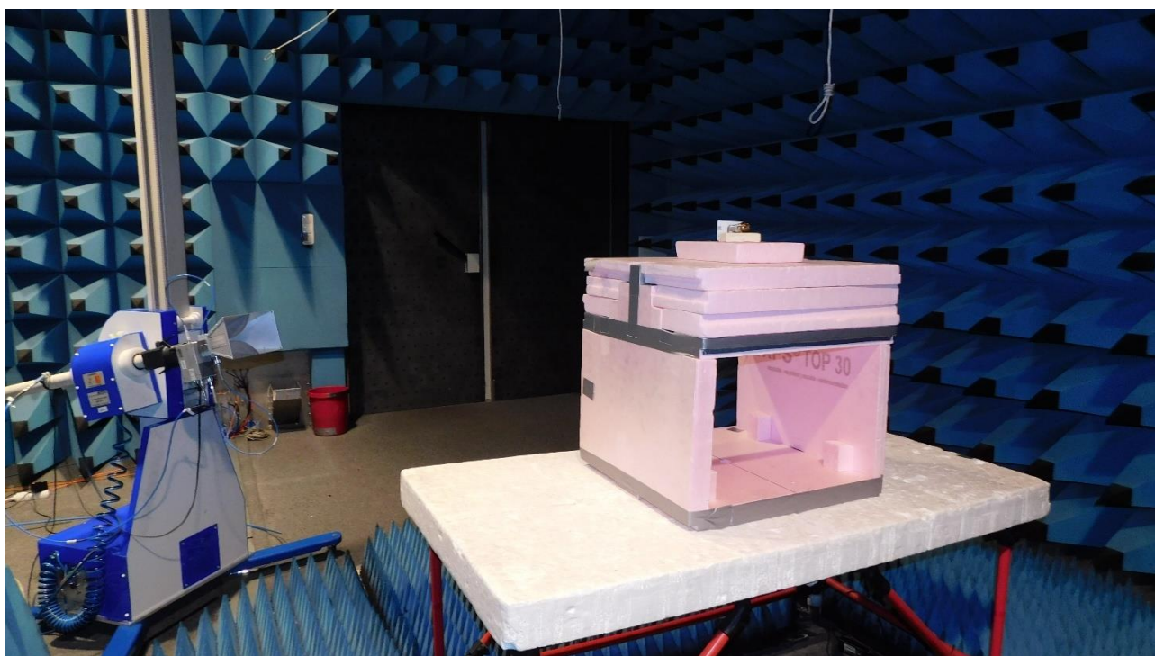
Picture 6: FS-SAC, radiated emission test 1 GHz – 17 GHz (rear view)
