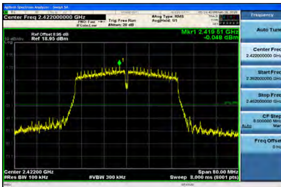
RF Conducted Spurious Emissions_11N40SISO_2422_Ant2
