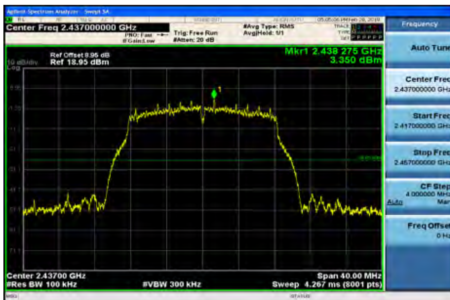
RF Conducted Spurious Emissions_11N20SISO_2437_Ant2
