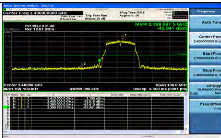
Band-edge for RF Conducted Emissions 11G_2462_Ant2
