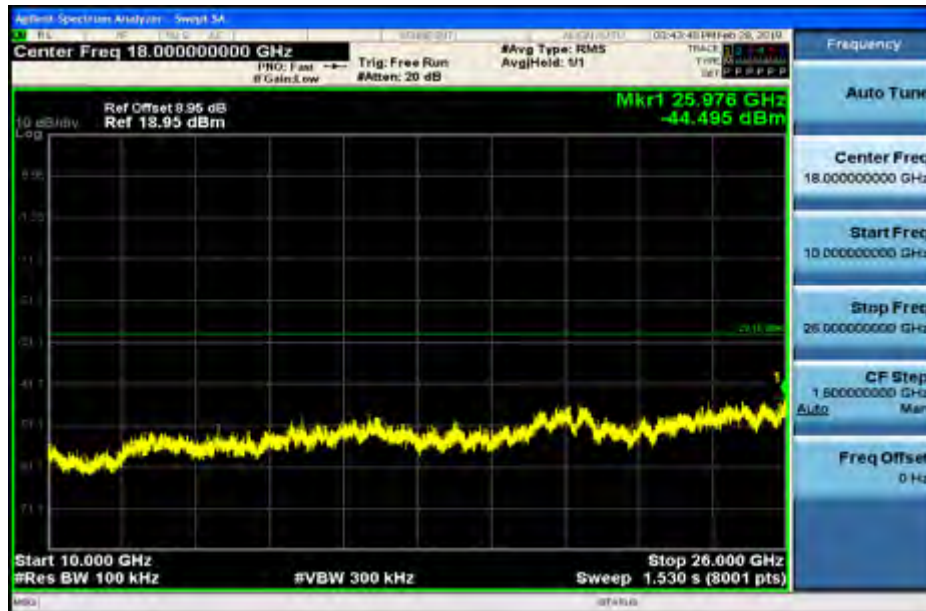
RF Conducted Spurious Emissions_11N40SISO_2422_Ant1
