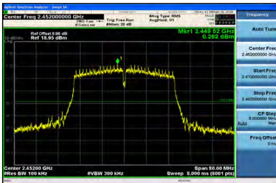
RF Conducted Spurious Emissions_11N40SISO_2452_Ant1
