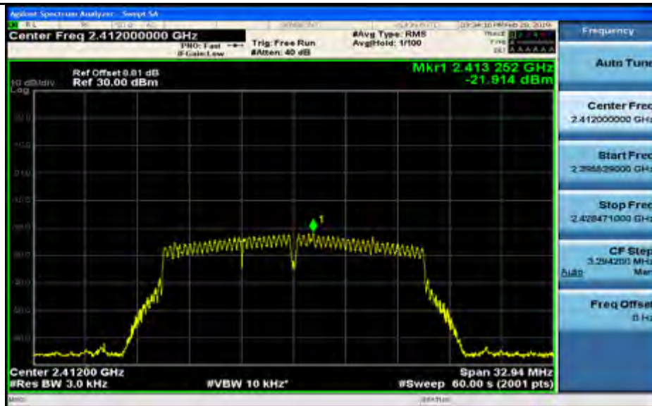
Maximum(average) power spectral density_11N20SISO_2437_Ant1
