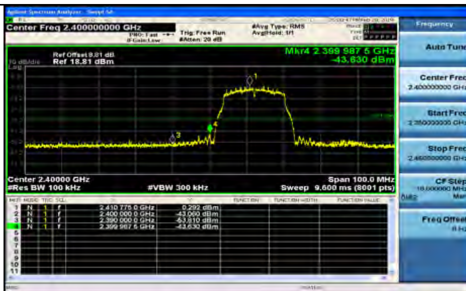
Band-edge for RF Conducted Emissions 11N20SISO_2462_Ant2
