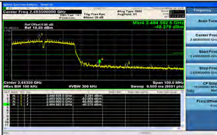
Band-edge for RF Conducted Emissions_11N40SISO_2452_Ant1
