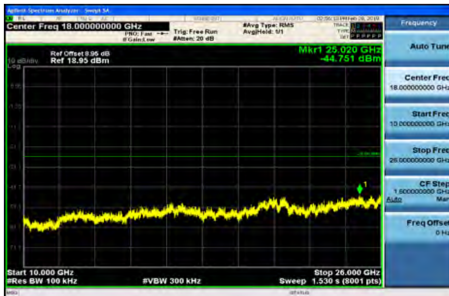
RF Conducted Spurious Emissions_11B_2462_Ant1
