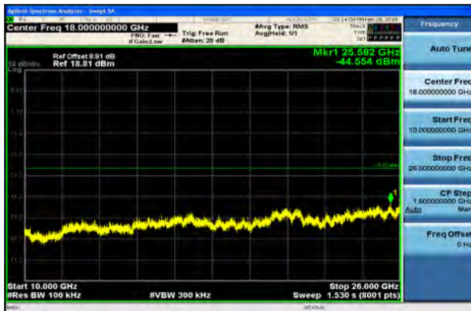
RF Conducted Spurious Emissions_11G_2437_Ant1
