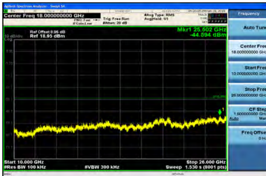
RF Conducted Spurious Emissions_11N40SISO_2437_Ant2
