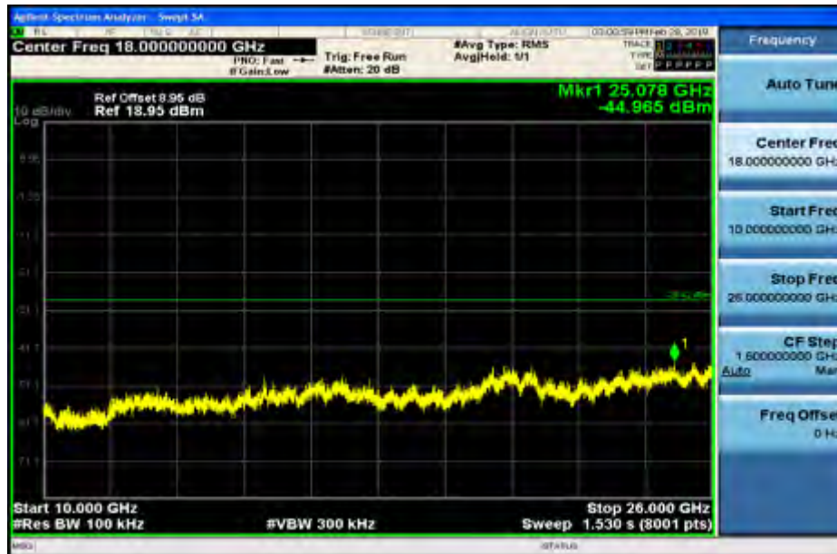
RF Conducted Spurious Emissions_11G_2412_Ant1
