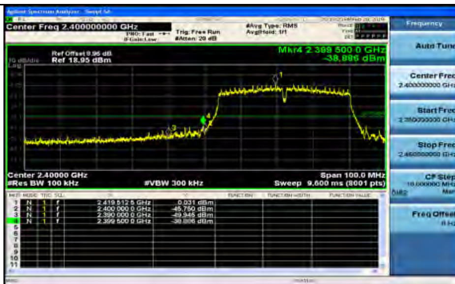
Band-edge for RF Conducted Emissions_11N40SISO_2452_Ant2
