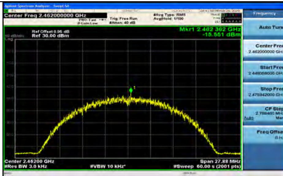
Maximum(average) power spectral density_11G_2412_Ant2
