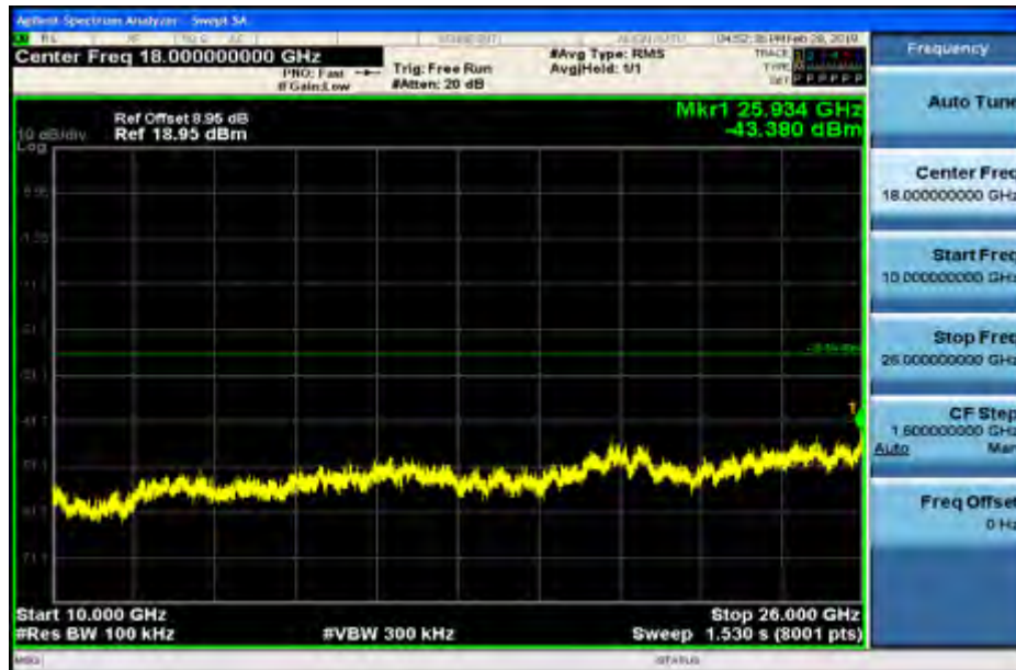
RF Conducted Spurious Emissions_11G_2462_Ant2
