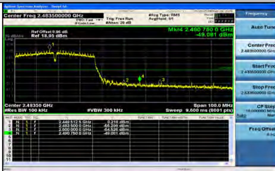
Band-edge for RF Conducted Emissions_11N40SISO_2452_Ant2
