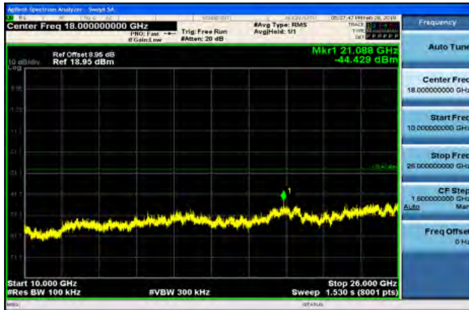
RF Conducted Spurious Emissions_11N40SISO_2452_Ant1
