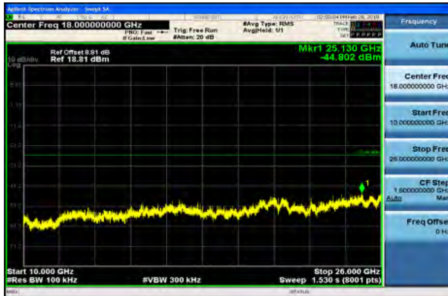
RF Conducted Spurious Emissions_11B_2437_Ant1
