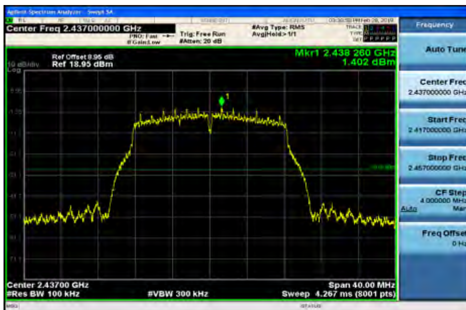
RF Conducted Spurious Emissions_11N20SISO_2437_Ant1
