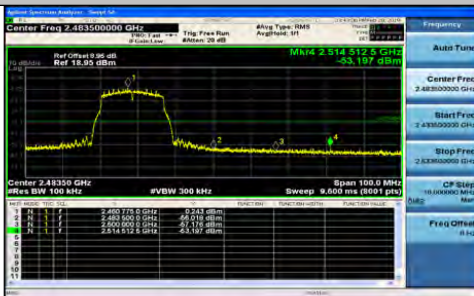
Band-edge for RF Conducted Emissions 11N40SISO 2422 Ant1
