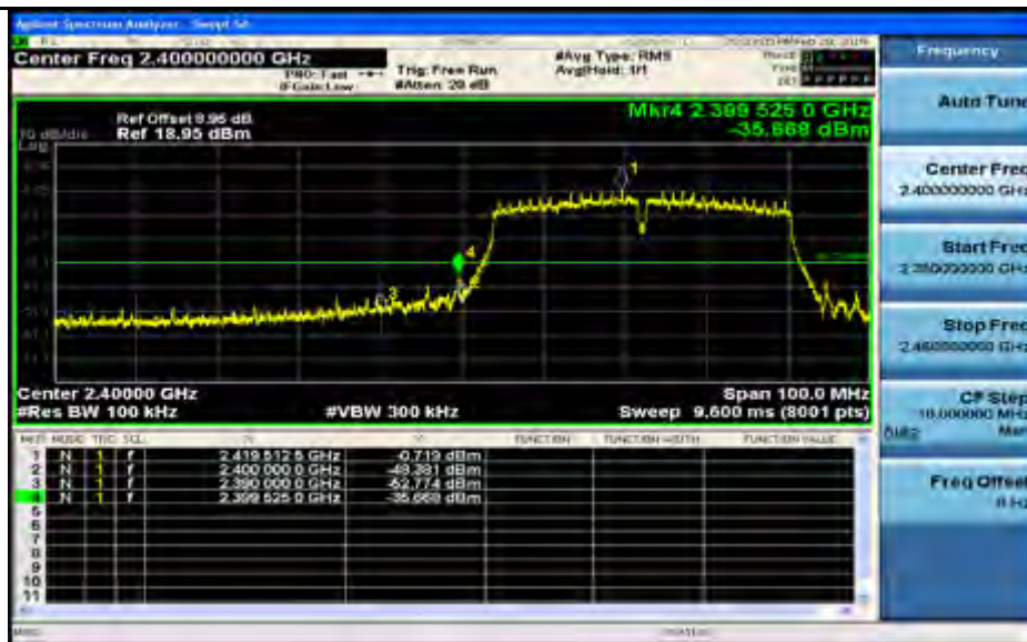
Band-edge for RF Conducted Emissions_11N40SISO_2452_Ant1
