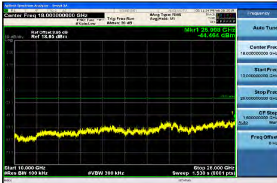
RF Conducted Spurious Emissions_11N40SISO_2422_Ant2
