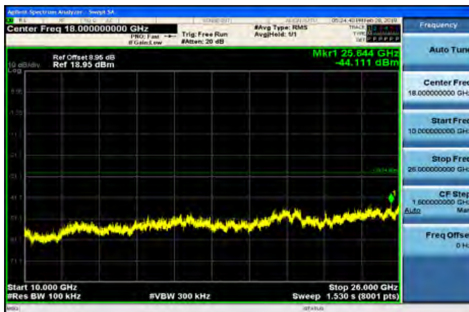
RF Conducted Spurious Emissions_11N40SISO_2452_Ant2
