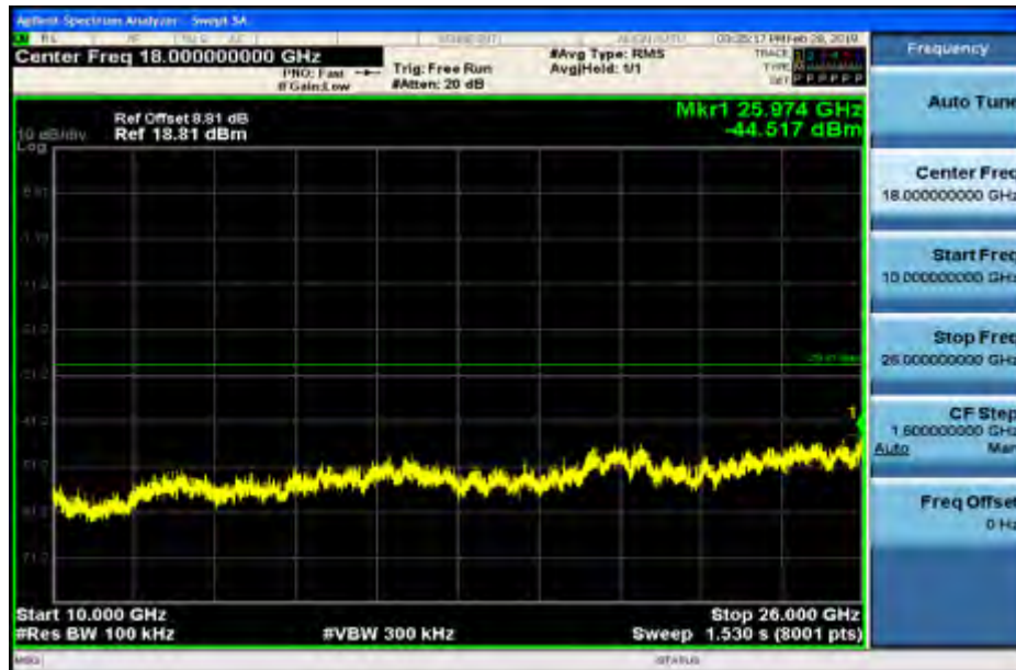
RF Conducted Spurious Emissions_11N20SISO_2437_Ant1
