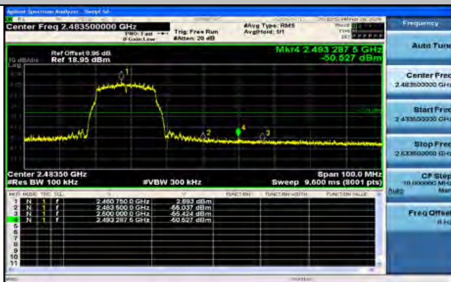
Band-edge for RF Conducted Emissions 11N40SISO 2422 Ant2
