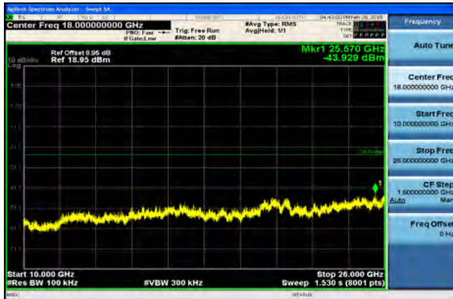
RF Conducted Spurious Emissions_11G_2412_Ant2
