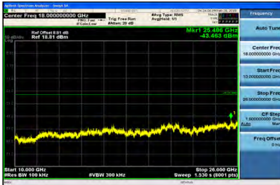
RF Conducted Spurious Emissions_11B_2437_Ant2
