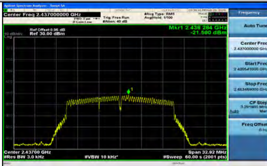
Maximum(average) power spectral density_11N20SISO_2462_Ant1
