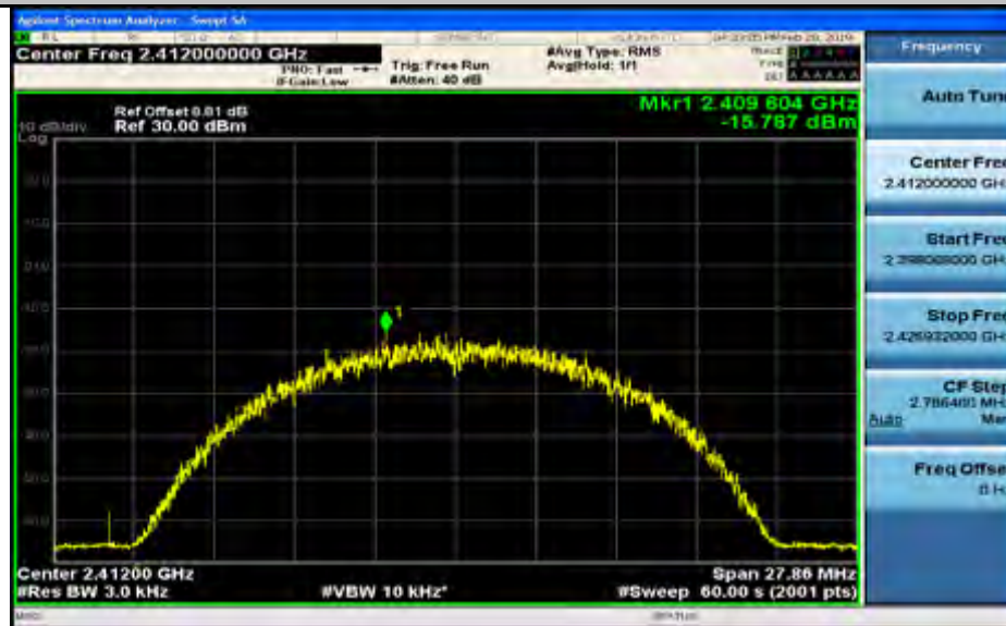
Maximum(average) power spectral density_11B_2437_Ant2
