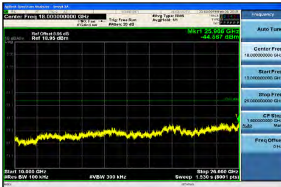
RF Conducted Spurious Emissions_11G_2462_Ant1
