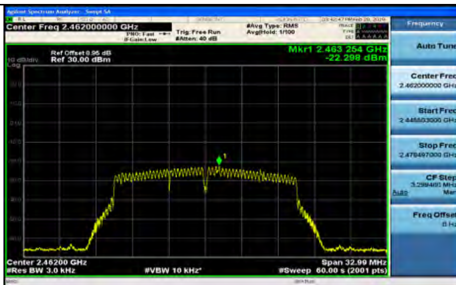
Maximum(average) power spectral density_11N40SISO_2422_Ant1
