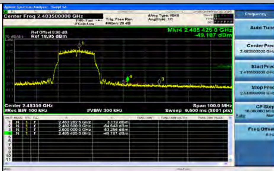
Band-edge for RF Conducted Emissions 11N20SISO 2412 Ant2
