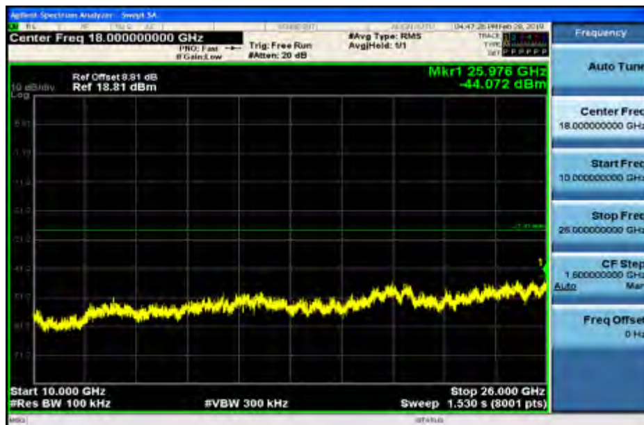
RF Conducted Spurious Emissions_11G_2437_Ant2
