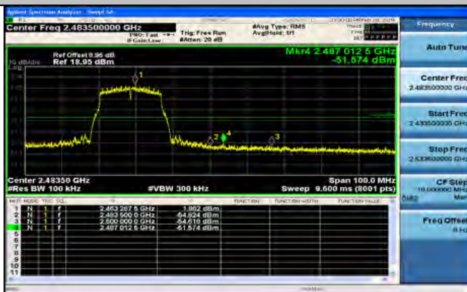
Band-edge for RF Conducted Emissions 11N20SISO 2412 Ant1
