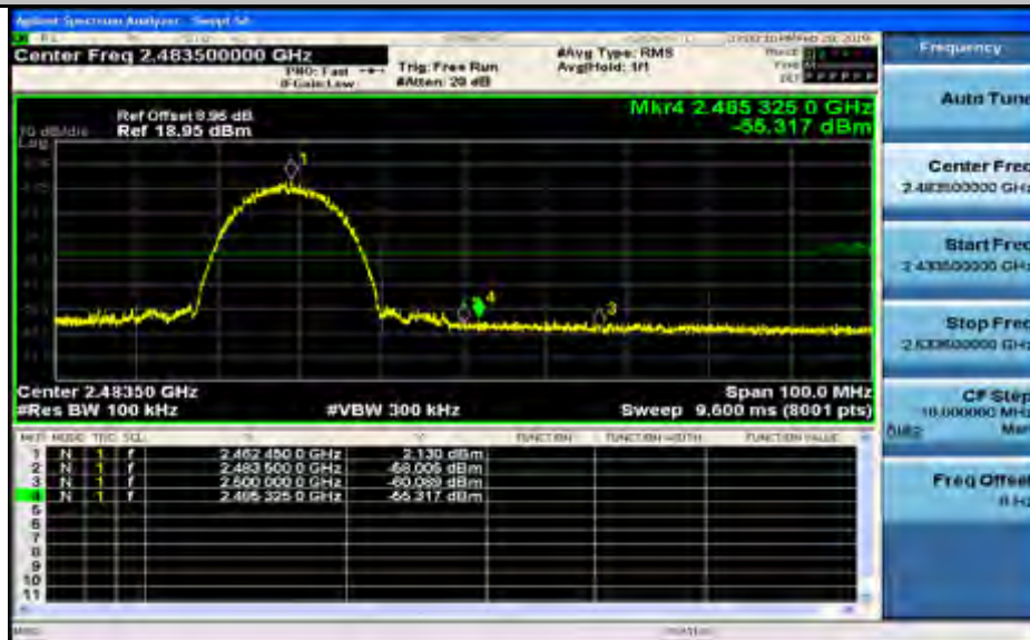
Band-edge for RF Conducted Emissions_11G_2412_Ant1
