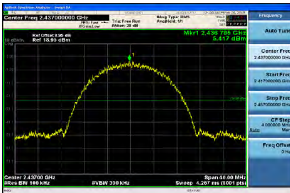
RF Conducted Spurious Emissions_11B_2437_Ant2
