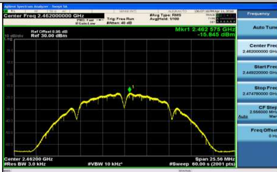
Maximum(average) power spectral density_11B_2462_Ant1
