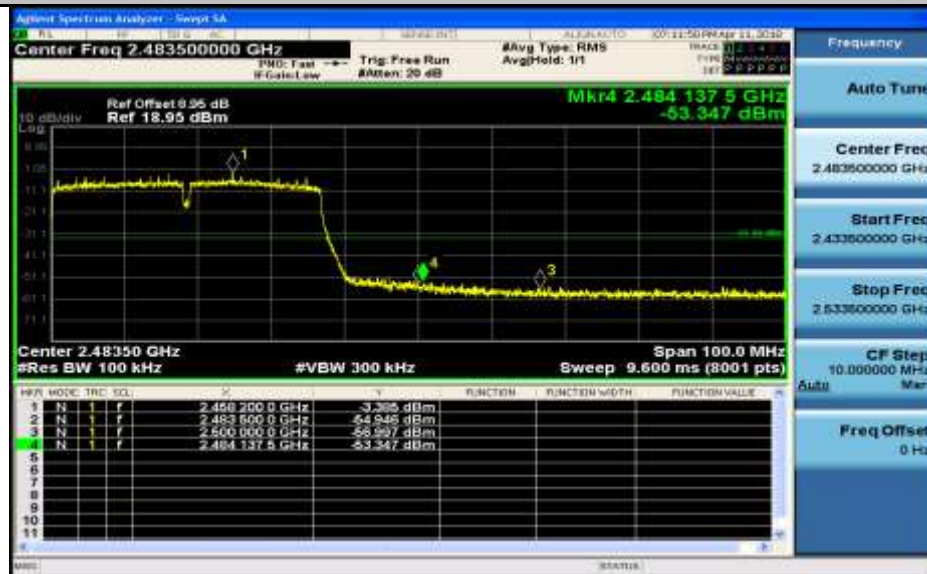
Band-edge for RF Conducted Emissions_11N40SISO_2452_Ant1
