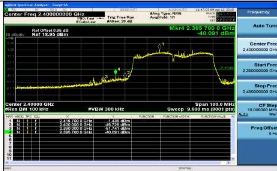
Band-edge for RF Conducted Emissions_11N40SISO_2452_Ant2
