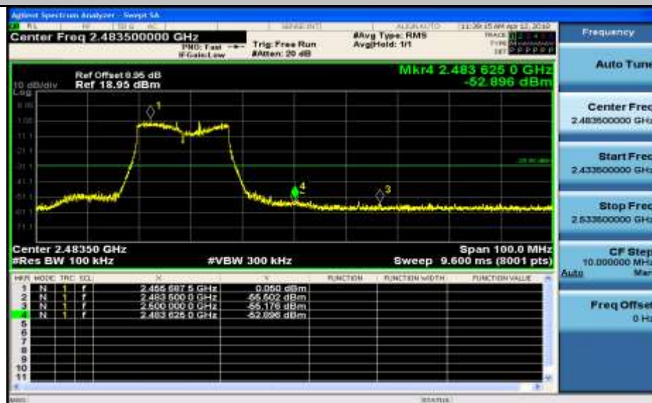
Band-edge for RF Conducted Emissions_11N20SISO_2462_Ant2
