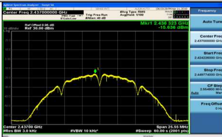
Maximum(average) power spectral density_11B_2462_Ant1
