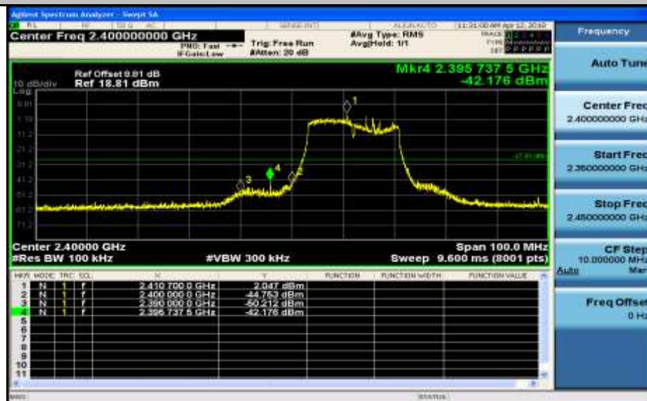
Band-edge for RF Conducted Emissions_11N20SISO_2462_Ant2
