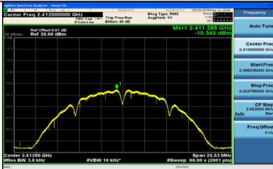
Maximum(average) power spectral density_11B_2437_Ant1
