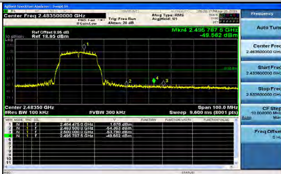
Band-edge for RF Conducted Emissions_11N20SISO_2412_Ant1
