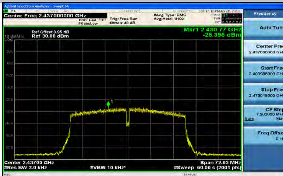
Maximum(average) power spectral density_11N40SISO_2452_Ant2
