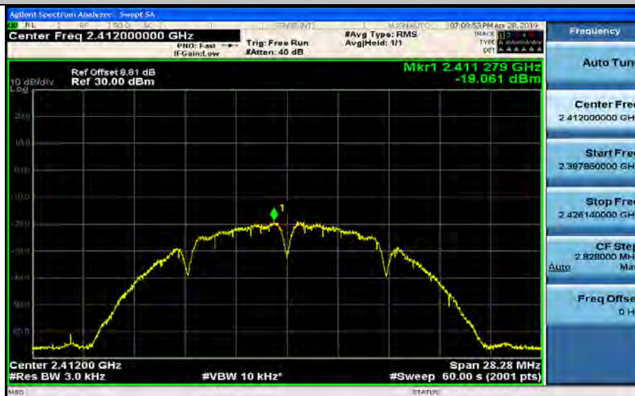
Maximum(average) power spectral density_11B_2437_Ant1
