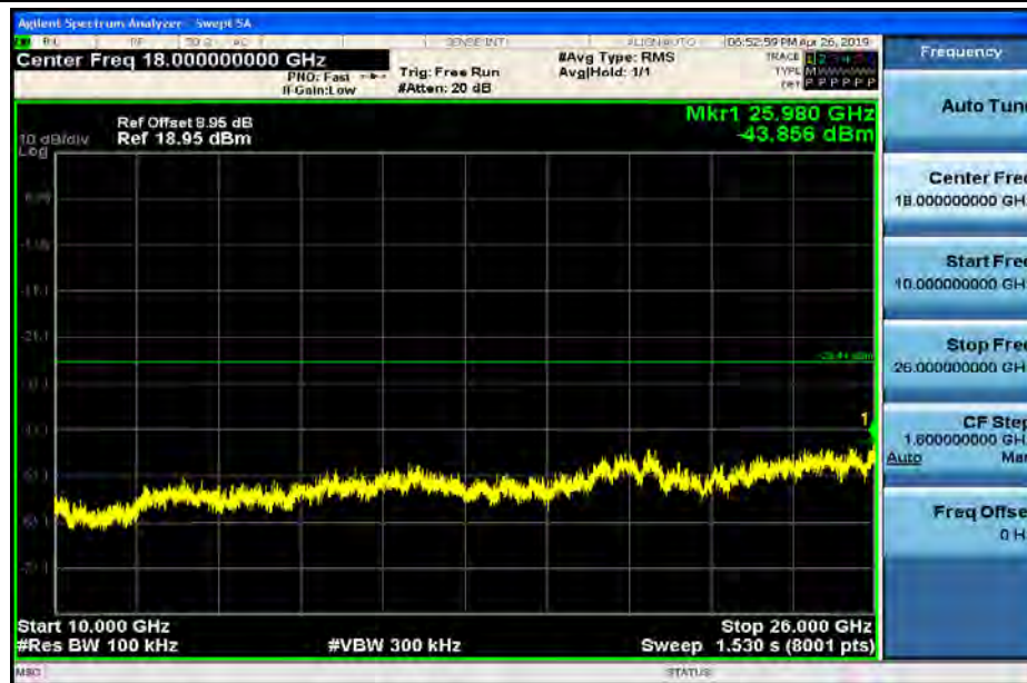
RF Conducted Spurious Emissions_11N20SISO_2412_Ant2
