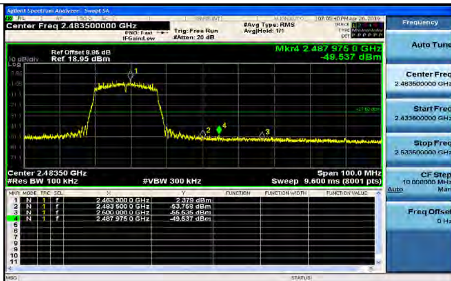
Band-edge for RF Conducted Emissions_11N40SISO_2422_Ant2
