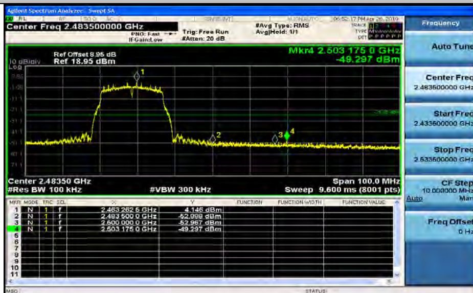
Band-edge for RF Conducted Emissions_11N20SISO_2412_Ant2
