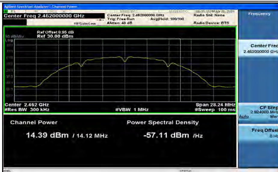
Maximum conducted (average) output power_11B_2462_Ant2
