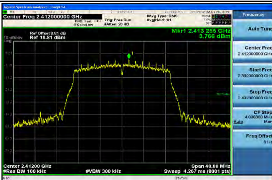
RF Conducted Spurious Emissions_11N20SISO_2412_Ant2
