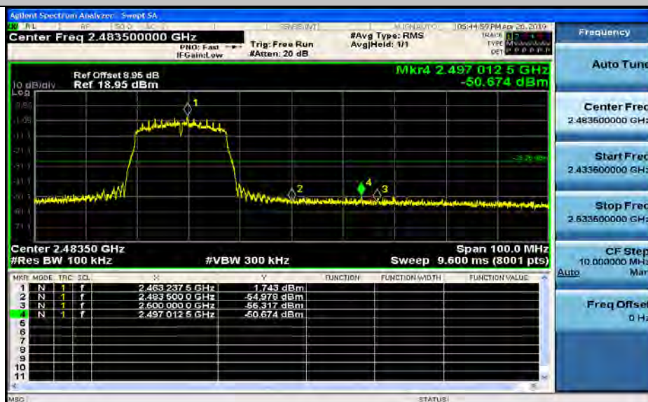
Band-edge for RF Conducted Emissions_11N20SISO_2462_Ant1
