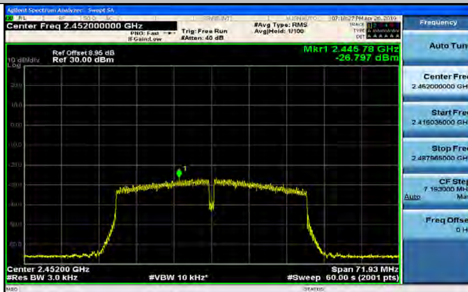
Maximum(average) power spectral density_11N40SISO_2452_Ant2
