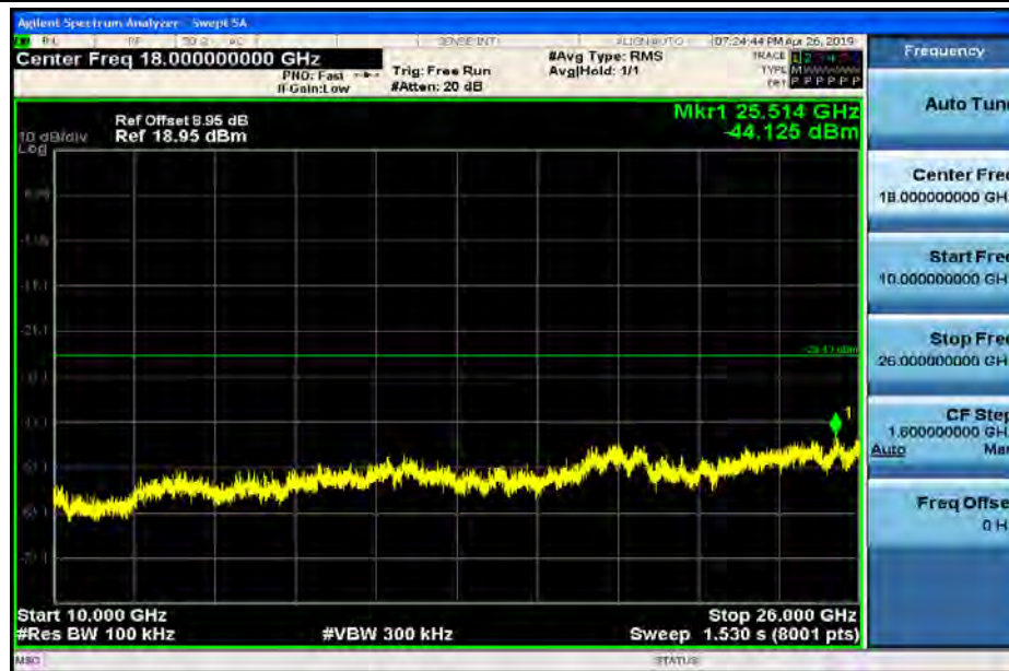
RF Conducted Spurious Emissions_11N20SISO_2462_Ant2
