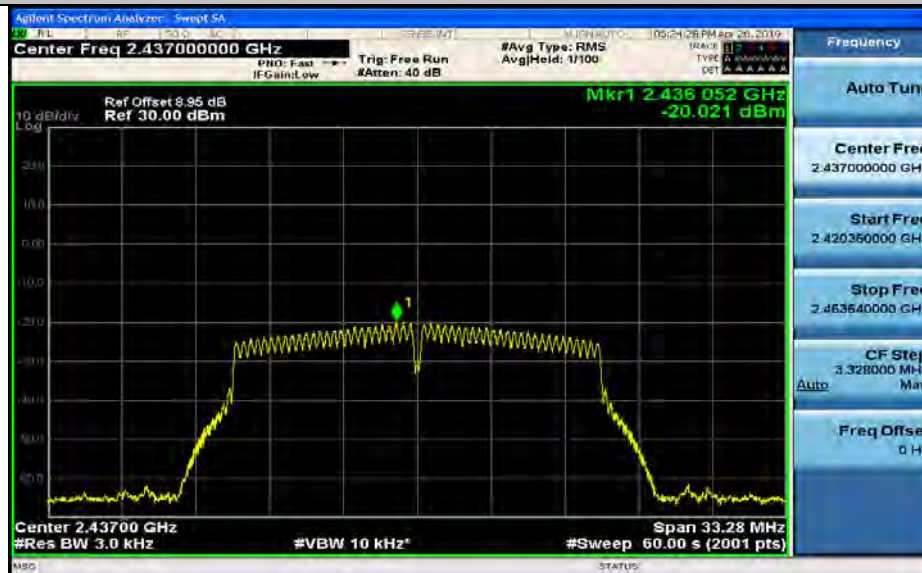
Maximum(average) power spectral density_11G_2462_Ant1
