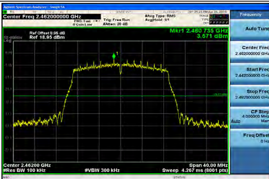
RF Conducted Spurious Emissions_11N20SISO_2462_Ant2
