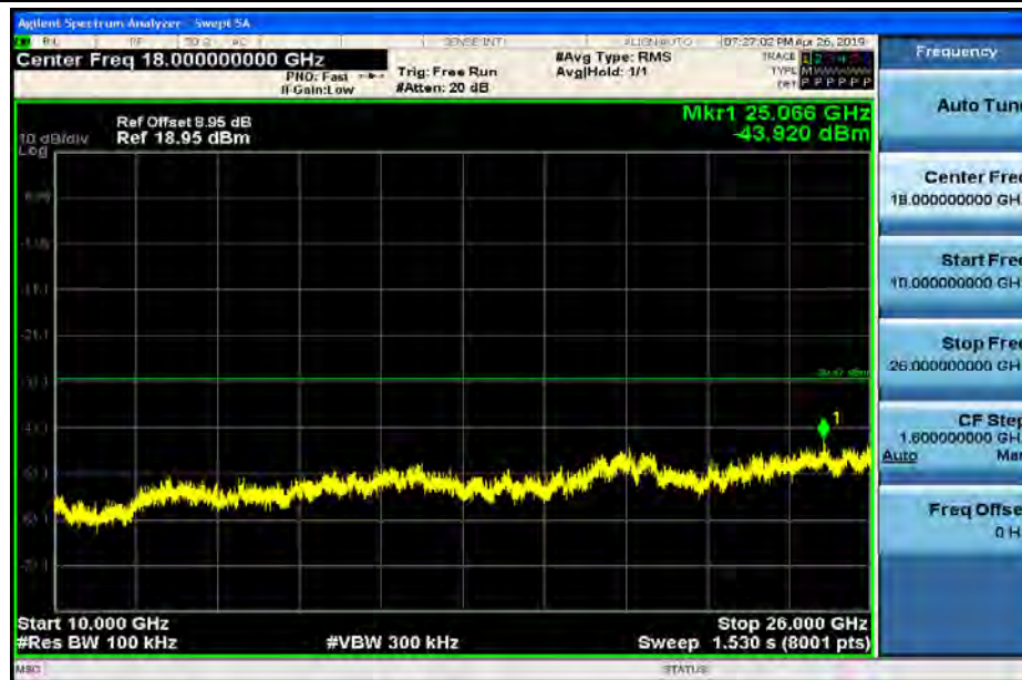
RF Conducted Spurious Emissions_11N40SISO_2437_Ant2
