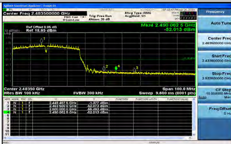
Band-edge for RF Conducted Emissions_11N40SISO_2452_Ant2
