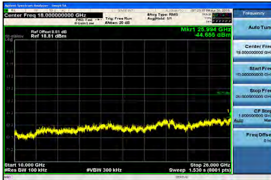
RF Conducted Spurious Emissions_11N20SISO_2437_Ant2
