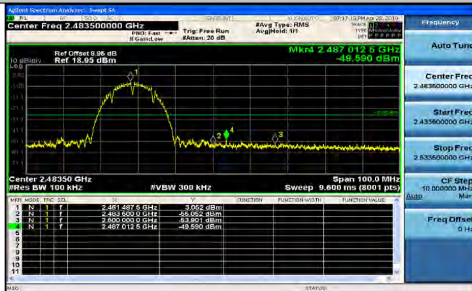
Band-edge for RF Conducted Emissions_11G_2412_Ant1
