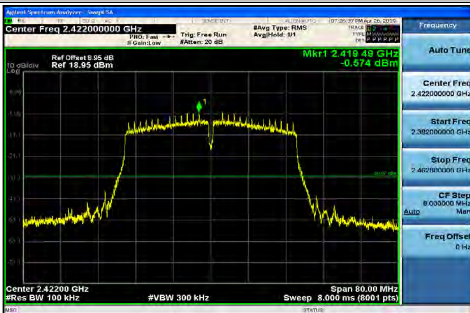
RF Conducted Spurious Emissions_11N40SISO_2422_Ant2
