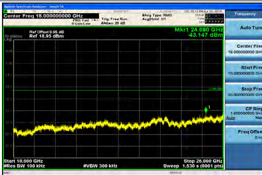
RF Conducted Spurious Emissions_11G_2412_Ant2
