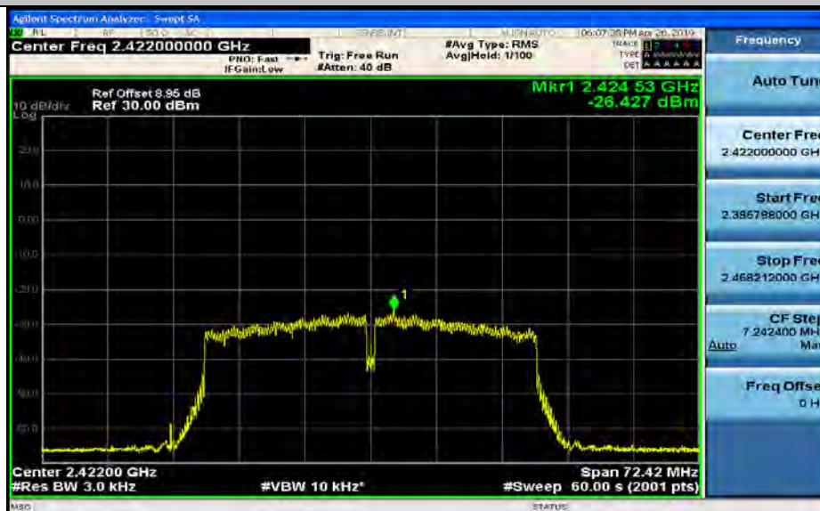
Maximum(average) power spectral density_11N40SISO_2437_Ant1
