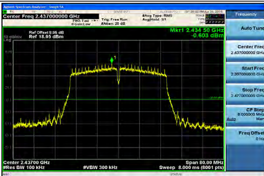
RF Conducted Spurious Emissions_11N40SISO_2437_Ant2
