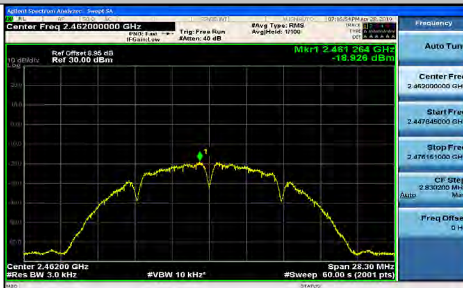
Maximum(average) power spectral density_11B_2462_Ant1
