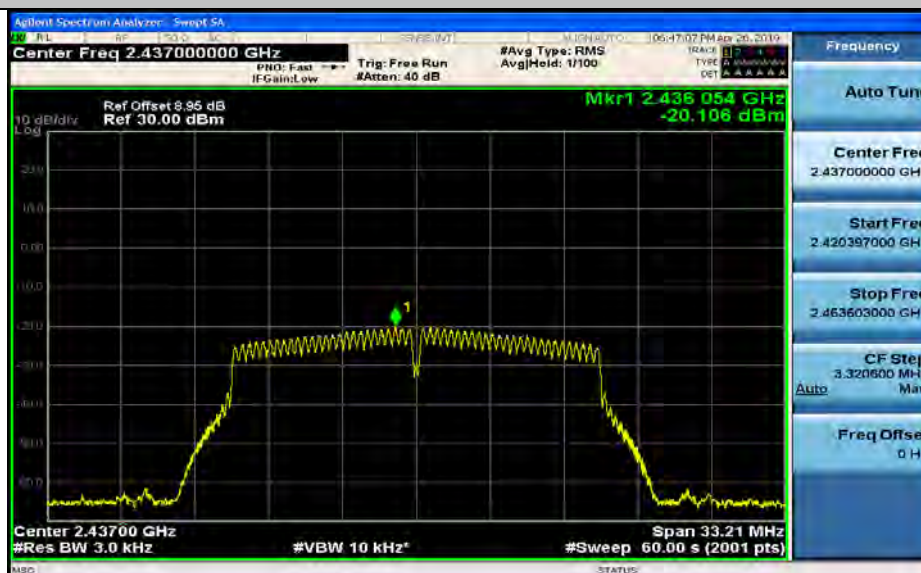
Maximum(average) power spectral density_11G_2462_Ant2
