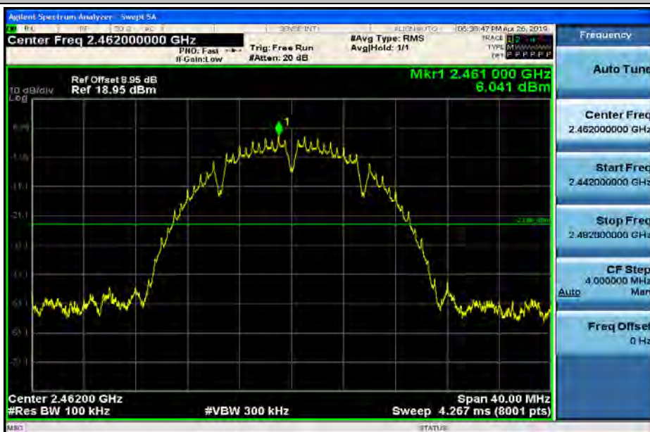
RF Conducted Spurious Emissions_11B_2462_Ant2
