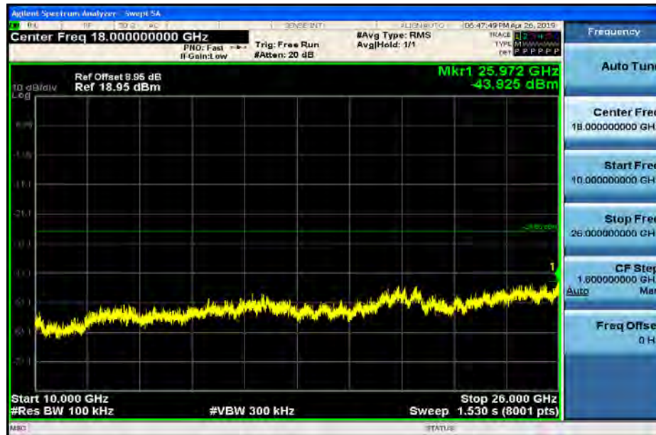
RF Conducted Spurious Emissions_11G_2462_Ant2
