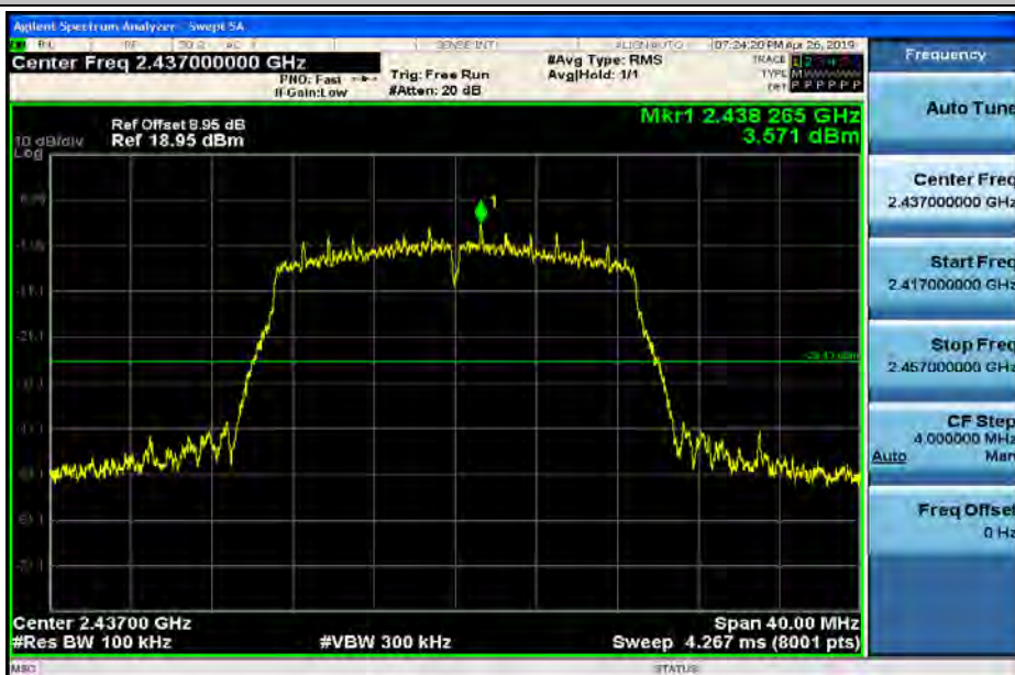
RF Conducted Spurious Emissions_11N20SISO_2437_Ant2
