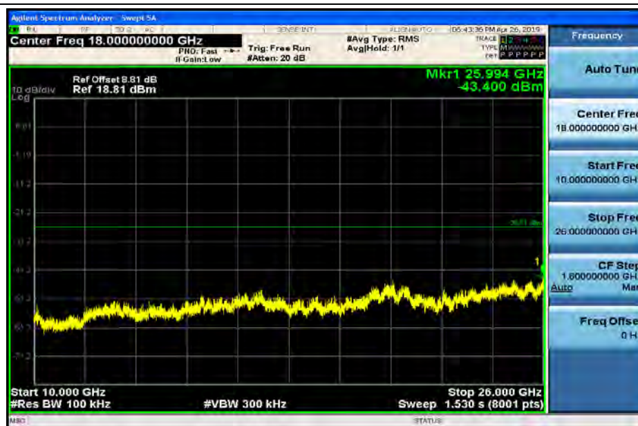
RF Conducted Spurious Emissions_11G_2437_Ant2
