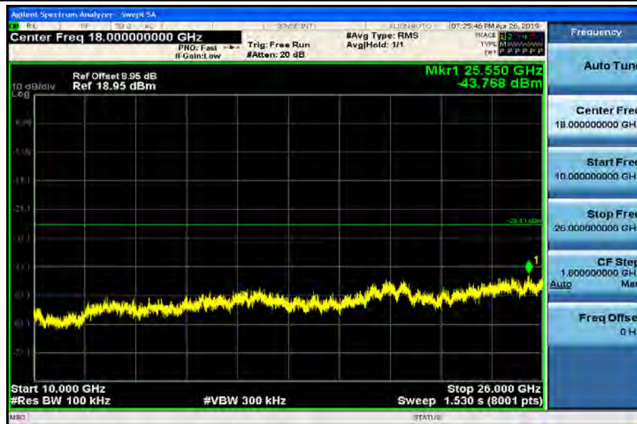
RF Conducted Spurious Emissions_11N40SISO_2422_Ant2
