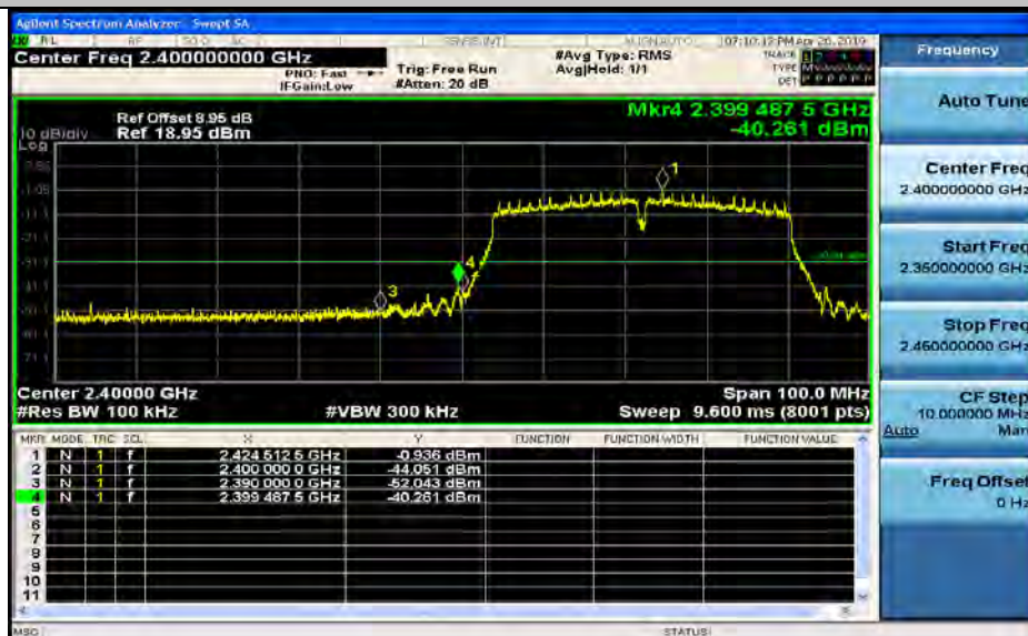
Band-edge for RF Conducted Emissions_11N40SISO_2452_Ant2
