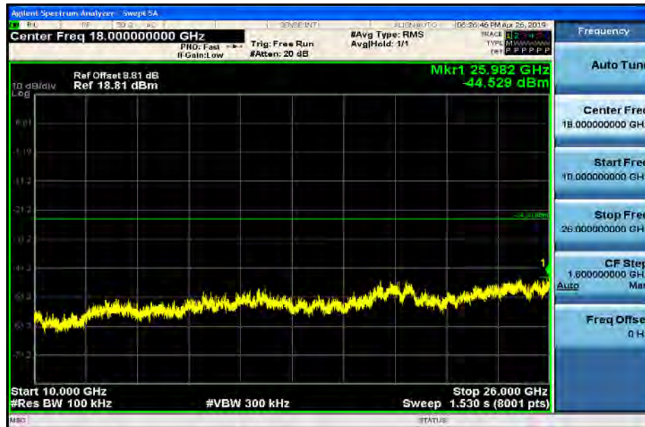
RF Conducted Spurious Emissions_11B_2437_Ant2
