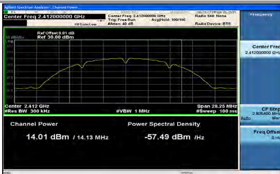
Maximum conducted (average) output power_11B_2437_Ant2
