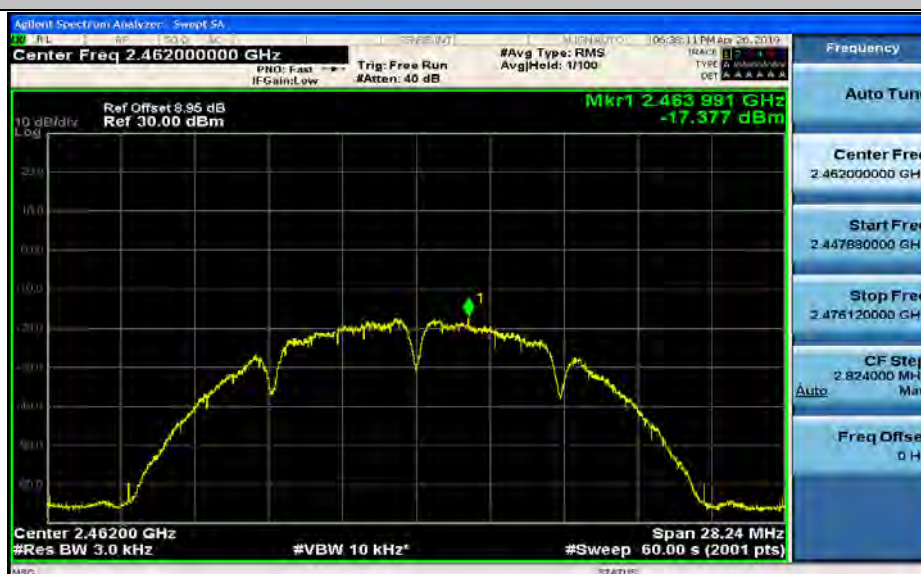
Maximum(average) power spectral density_11B_2462_Ant2
