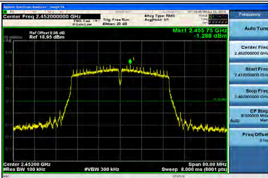
RF Conducted Spurious Emissions_11N40SISO_2452_Ant2
