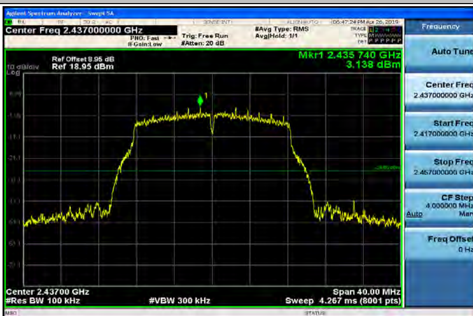
RF Conducted Spurious Emissions_11G_2437_Ant2
