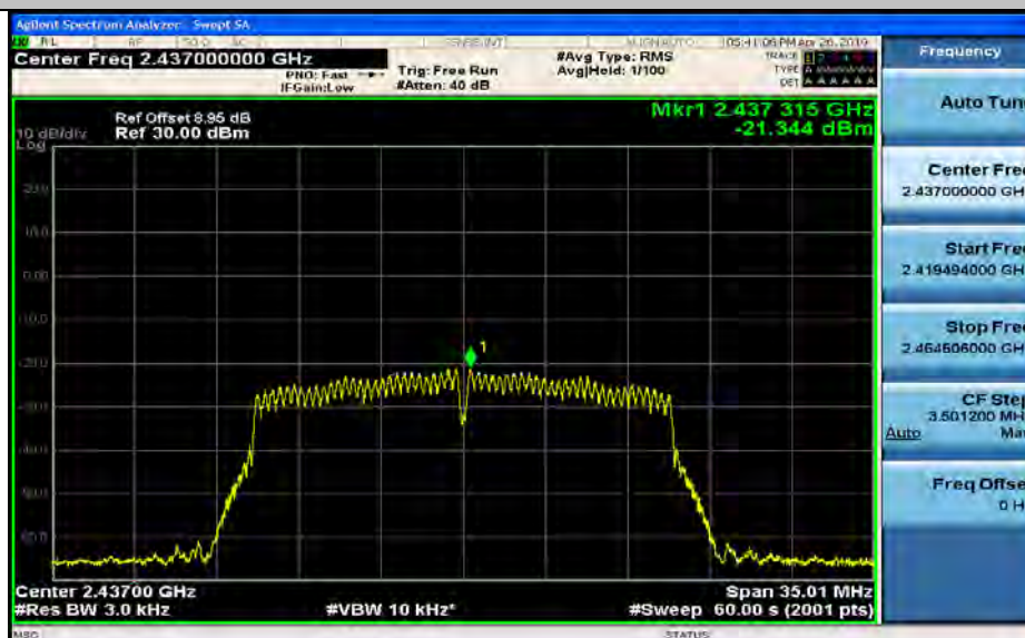
Maximum(average) power spectral density_11N20SISO_2462_Ant1
