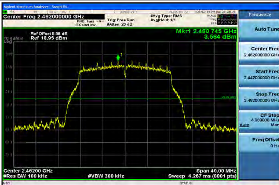
RF Conducted Spurious Emissions_11G_2462_Ant2
