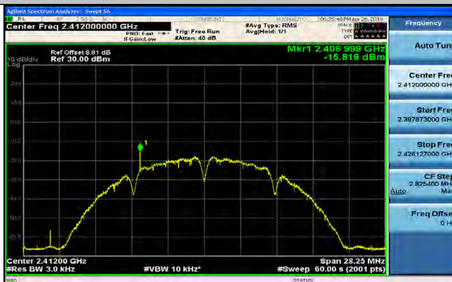
Maximum(average) power spectral density_11B_2437_Ant2
