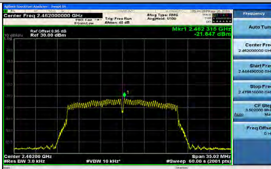
Maximum(average) power spectral density_11N20SISO_2462_Ant1
