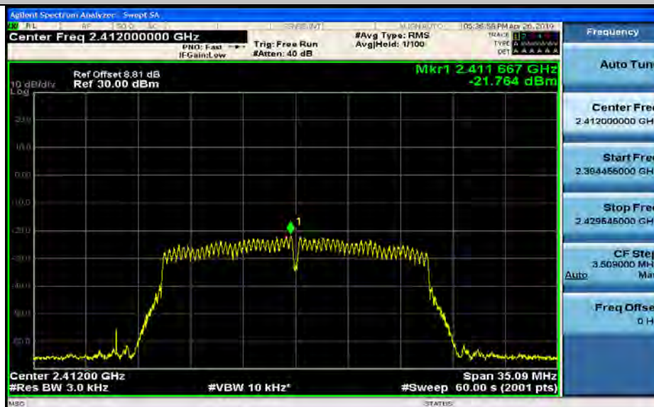
Maximum(average) power spectral density_11N20SISO_2437_Ant1
