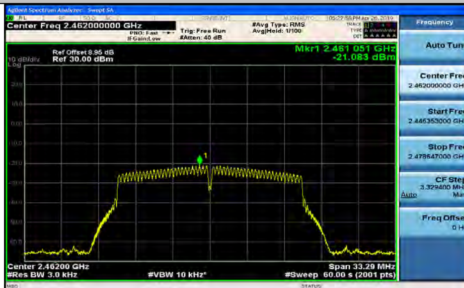
Maximum(average) power spectral density_11G_2462_Ant1
