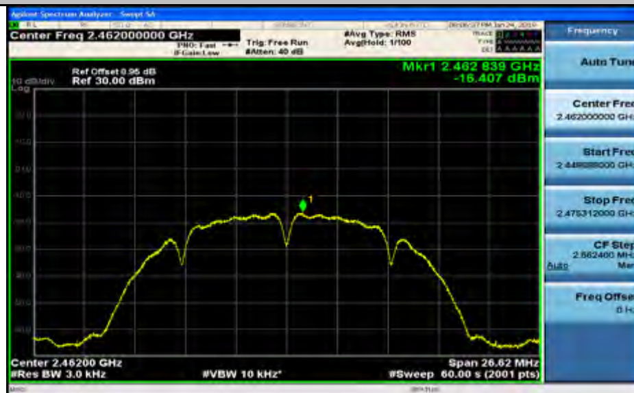
Maximum(average) power spectral density_11B_2462_Ant2
