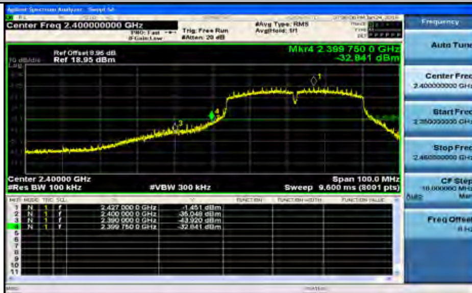
Band-edge for RF Conducted Emissions_11N40SISO_2452_Ant1
