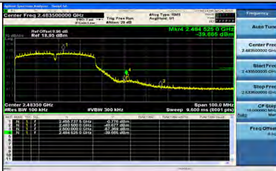
Band-edge for RF Conducted Emissions_11N40SISO_2452_Ant1
