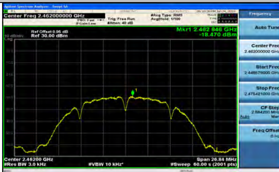
Maximum(average) power spectral density_11B_2462_Ant1
