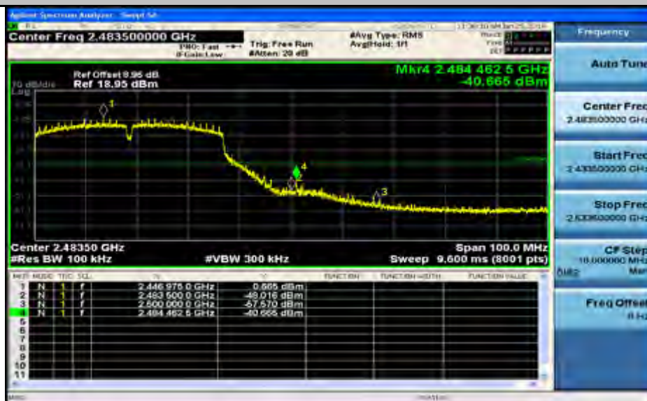
Band-edge for RF Conducted Emissions_11N40ISO_2452_Ant2
