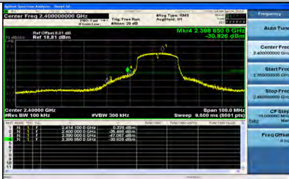
Band-edge for RF Conducted Emissions_11N20SISO_2462_Ant1
