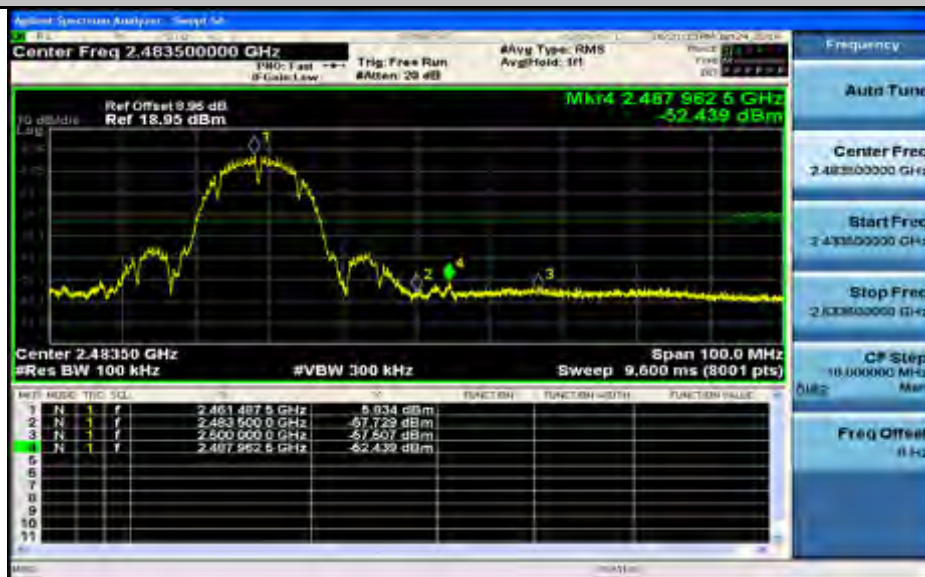
Band-edge for RF Conducted Emissions_11G_2412_Ant1
