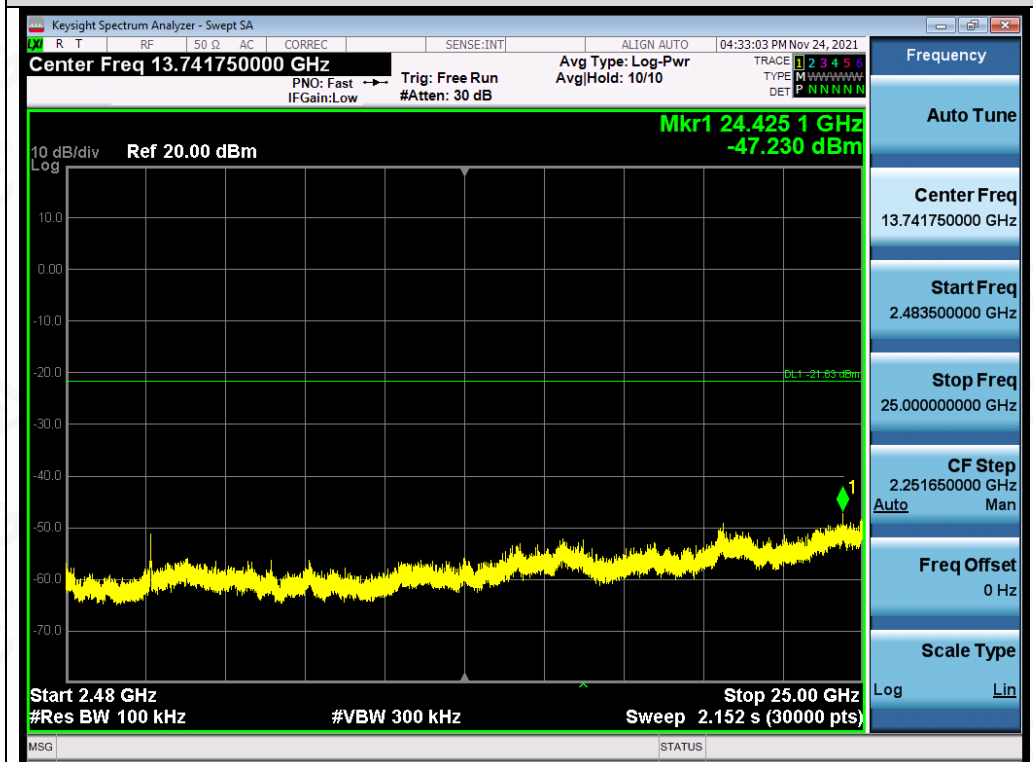
Test_Graph_802.11g_ANT1_2437_6Mbps_Higher Band Emissions
