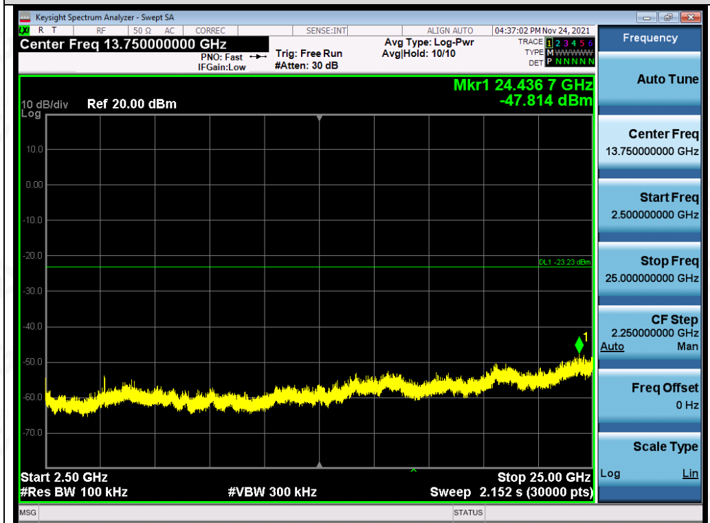
Test_Graph_802.11g_ANT1_2462_6Mbps_Higher Band Emissions
