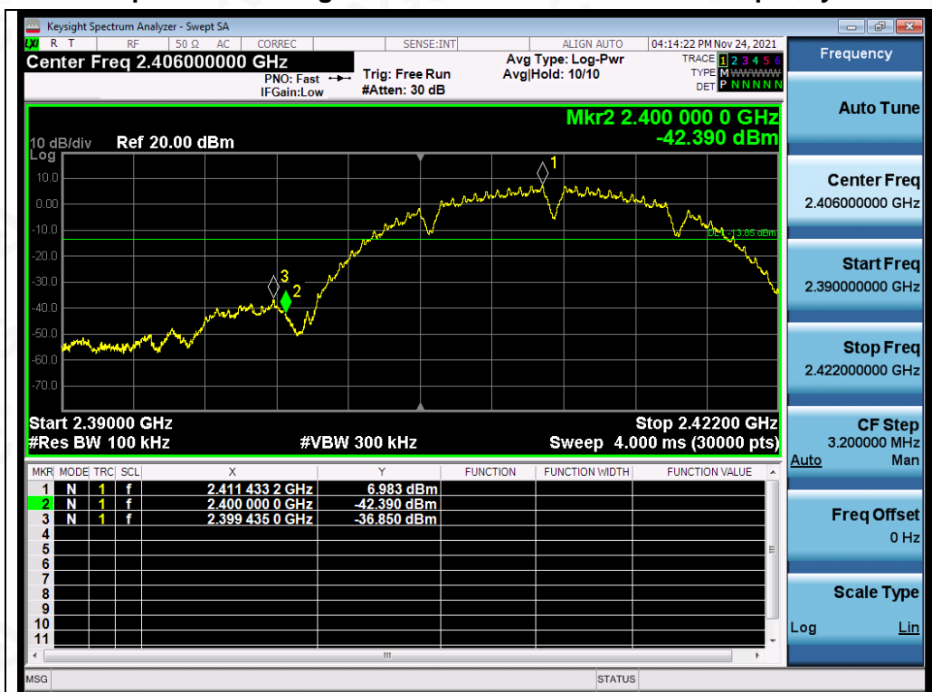
Test_Graph_802.11b_ANT1_2412_1Mbps_Lower Band Edge Emissions
