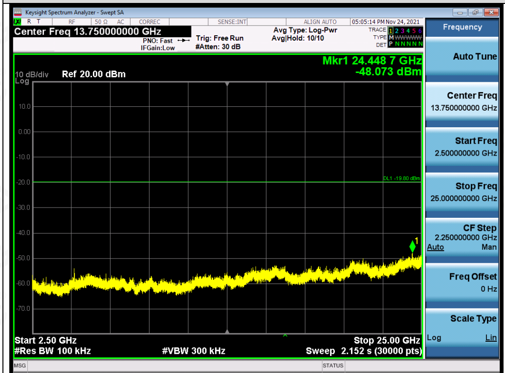
Test_Graph_802.11n20_ANT1_2462_MCS0_Higher Band Emissions
