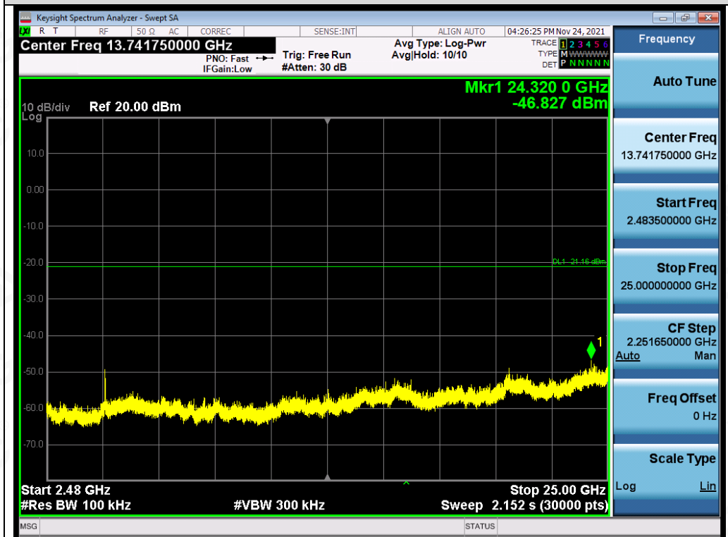
Test_Graph_802.11g_ANT1_2412_6Mbps_Higher Band Emissions
