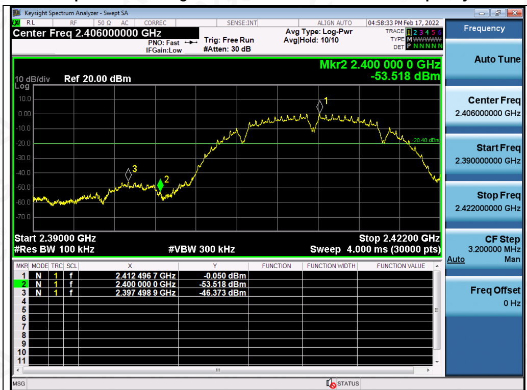
Test_Graph_802.11b_ANT1_2412_1Mbps_Lower Band Edge Emissions
