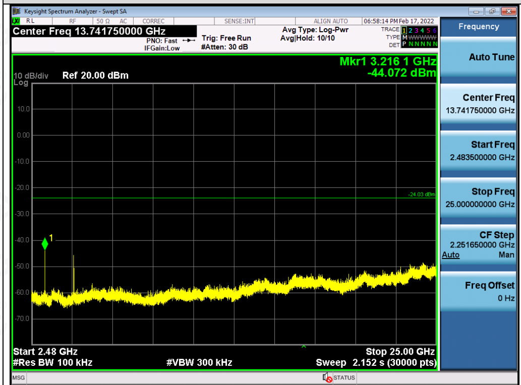
Test_Graph_802.11n20_ANT1_2412_MCS0_Higher Band Emissions
