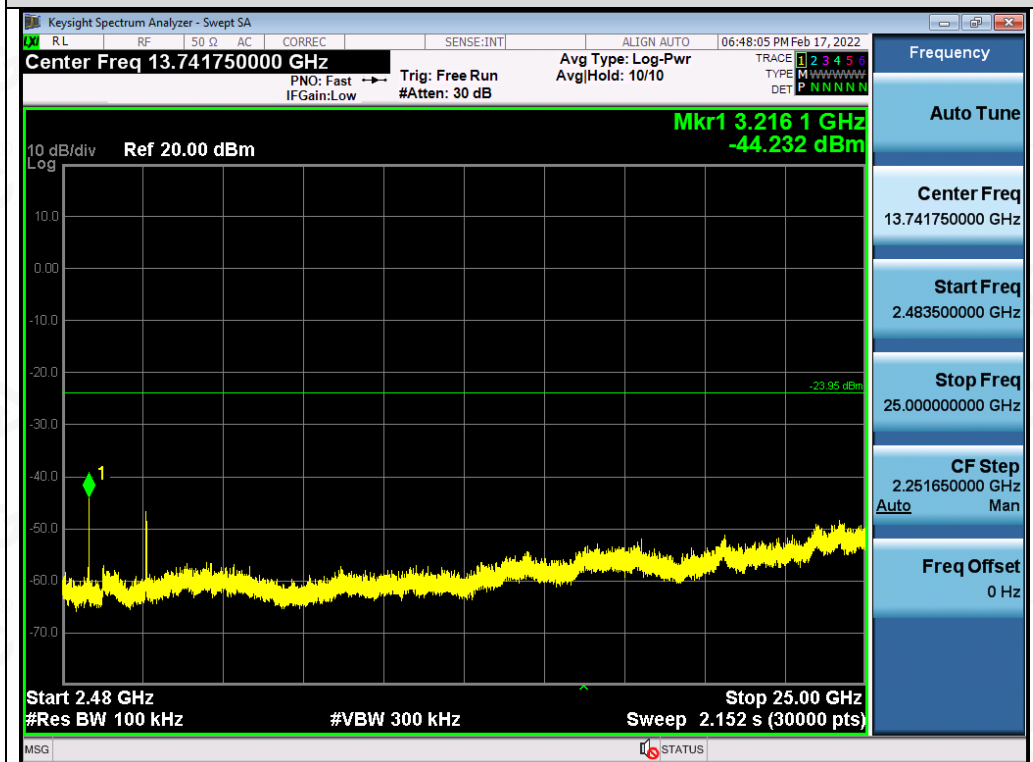
Test_Graph_802.11g_ANT1_2412_6Mbps_Higher Band Emissions
