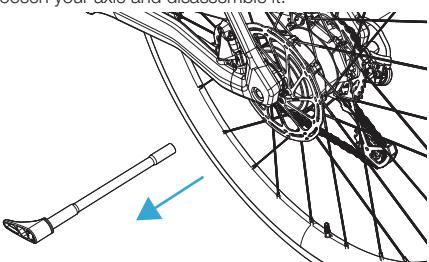
4. Slide the wheel out of the frame. Ensure you give room to the wheel by pressing the rear derailleur away from the cassette.
