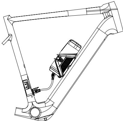
The Range Extender carries 171Wh in addition and allows you to increase your range drastically, while only adding 1.1Kg of extra weight to the system. This will upgrade your total capacity by 77% when added to the IX250 battery and 53% when added to the IX350 battery. The new designed holder for the e185 Range Extender follows the design, size and mounting points of a regular bottle cage and can therefore also be used to carry a regular bottle when the Range Extender is not used.
