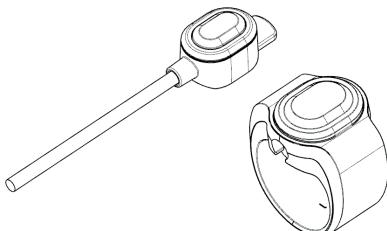
By pressing the e-Shifters, whether briefly or for longer, different commands are sent to the system. A maximum of 2 e-Shifters per eBike can be installed (left and right).
