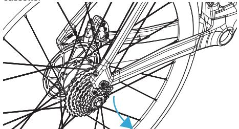
5. Ensure to not damage the frame with the disc rotor when sliding the wheel out of the frame.
