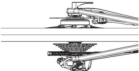
3. Carefully slide the rear wheel into the dropouts. Please ensure that the motor connector is facing upwards and is aligned with the dropout. Once the wheel sits smoothly in the dropouts, guide the axle through the motor and tighten it to the frame manufacturers recommendations. Once the axle is tight, the motor is automatically connected to the rest of the system.
