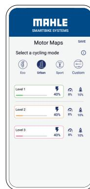
The system also features a CUSTOM mode. The CUSTOM mode will allow you to customize each of the assist levels (1 to 3) by adjusting peak power, acceleration, and reactivity.
