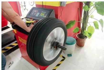
Step 6: Inflate the tires, check whether there is air leakage by the soap water, and do dynamic balance test after installation on the vehicle. Paste warning labels and the installation process is finished.
