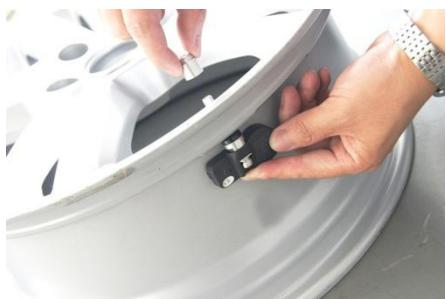
Step 4: Install the fixing nut by hand in advance.
