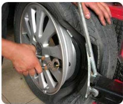
Step 1: Remove the tire and the inflating valve.
