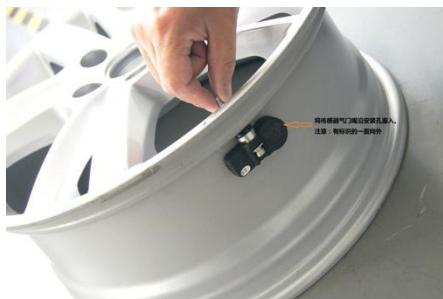
Step 2: Remove the dust cap, the fixing nut and the washer. Install the sensor into the installation hole of the inflating valve.
