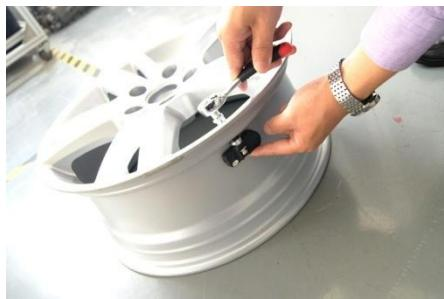
Step 5: Use 11# box spanner to tighten the fixing nut with torque force 4.0 - 5.0 Nm.
