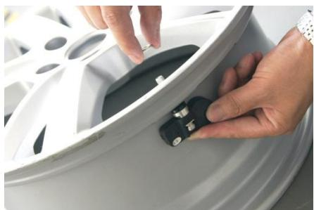
Step 3: Install the washer.
