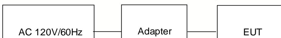
Operation of EUT during Radiation and Above1GHz Radiation testing:
