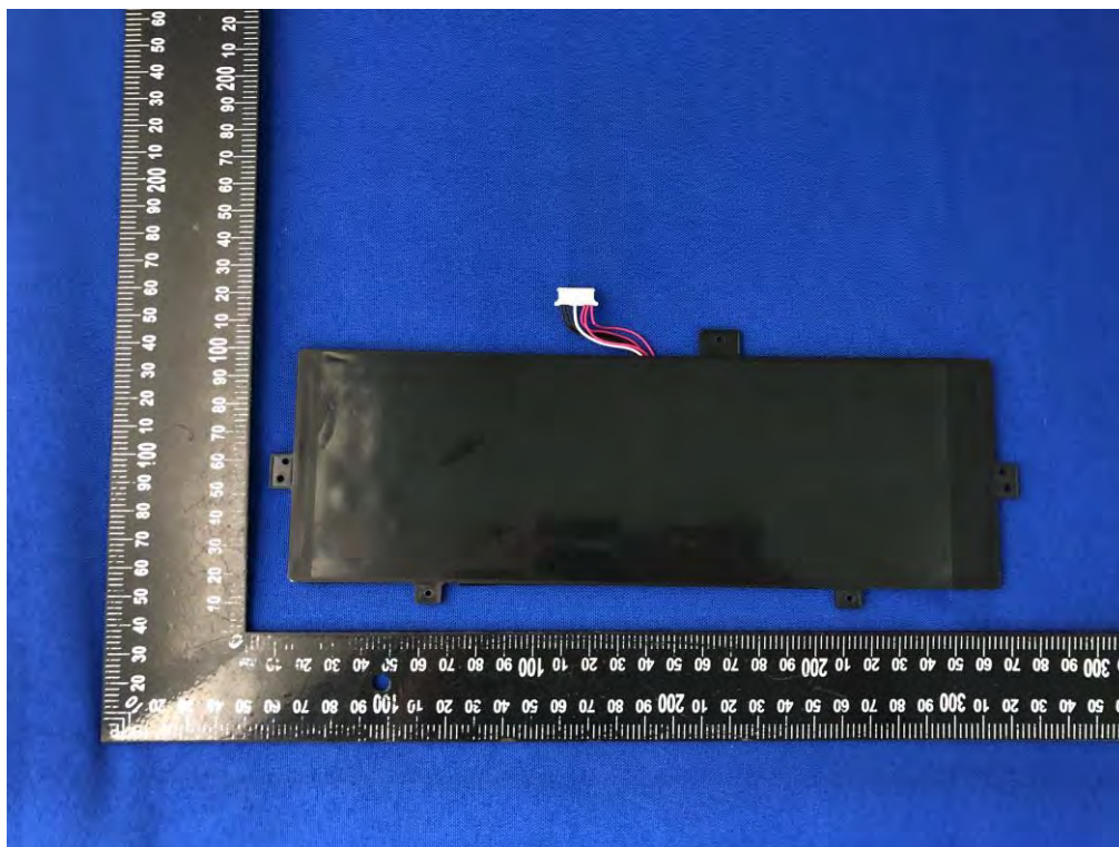
Battery Photo (REAR)
