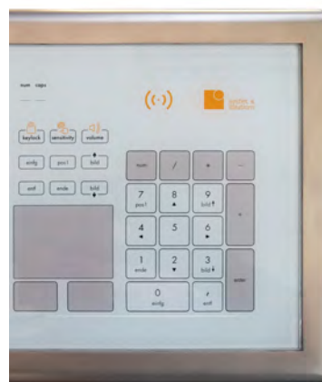
Fig. 8: RFID reader position on an TNGR keyboard
