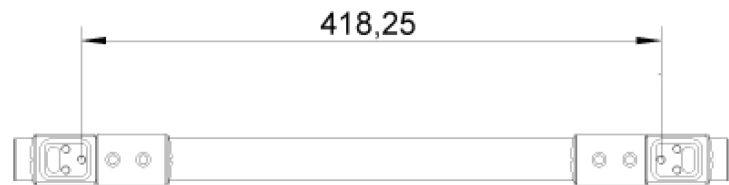
Fig. 22: Drill hole specification
