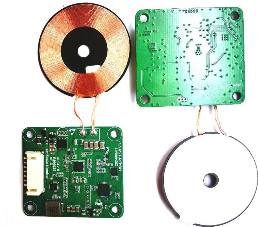
3. The shape of the transmitter board is as shown in the following picture. When using, it only needs to connect the usb-c interface. Note that the input voltage is qc3.0 adapter or 5-9vdc power supply. Blue green LED will flash when power on:
