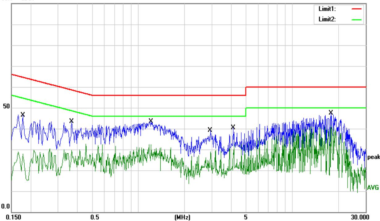
Note: The input of ANU-C1802 (5V/2A, 9V/2A), ANU-C1802-1 (5V/2A), ANU-C1802-2 (5V/2A, 9V/2A), ANU-C1802-3 (5V/2A, 9V/2A) all have tested, the worst case is ANU-C1802 (9V/2A), only show the worst case.
