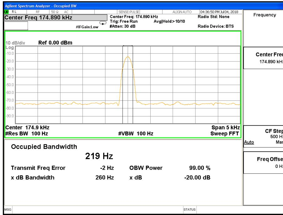
Note: The input of ANU-C1802 (5V/2A, 9V/2A), ANU-C1802-1 (5V/2A), ANU-C1802-2 (5V/2A, 9V/2A), ANU-C1802-3 (5V/2A, 9V/2A) all have tested, the worst case is ANU-C1802 (9V/2A), only show the worst case.
