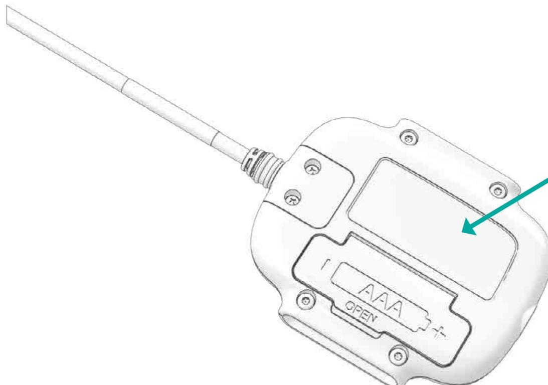
**2** Insert or scan the serial number located on the wrist device
