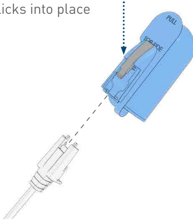
**2** Attach new sticker to the chest sensor by peeling off the cover on one side of the sticker
