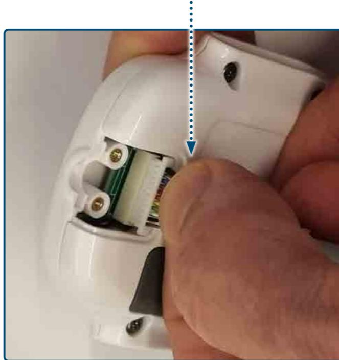
**3** Connect a new finger probe cable by gently inserting the connector back into the wrist module until a click is heard.
