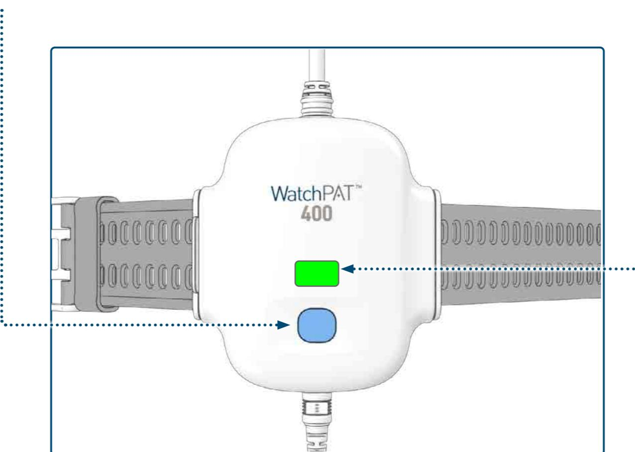
**2** The LED will flash green for one second to indicate the self-diagnostic tests has started
