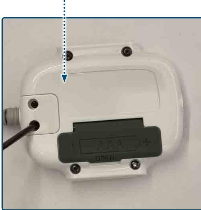
**2** Carefully disconnect the cable from the connector by pulling out the cable
