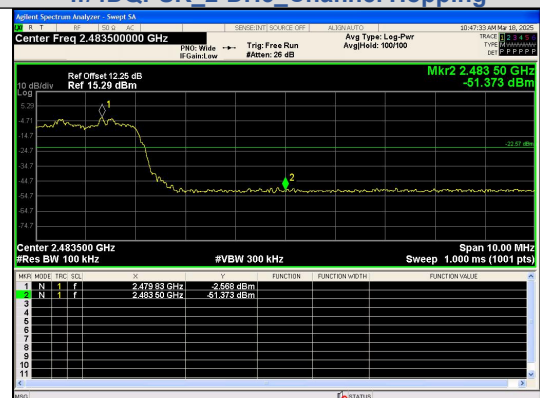
Out of Band Emission(Right) \pi/4 DQPSK_2-DH5_Channel Hopping
