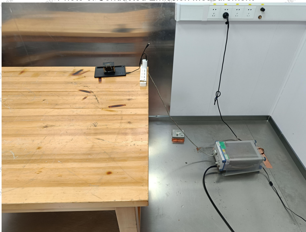
Photo of Conducted Emission Measurement
