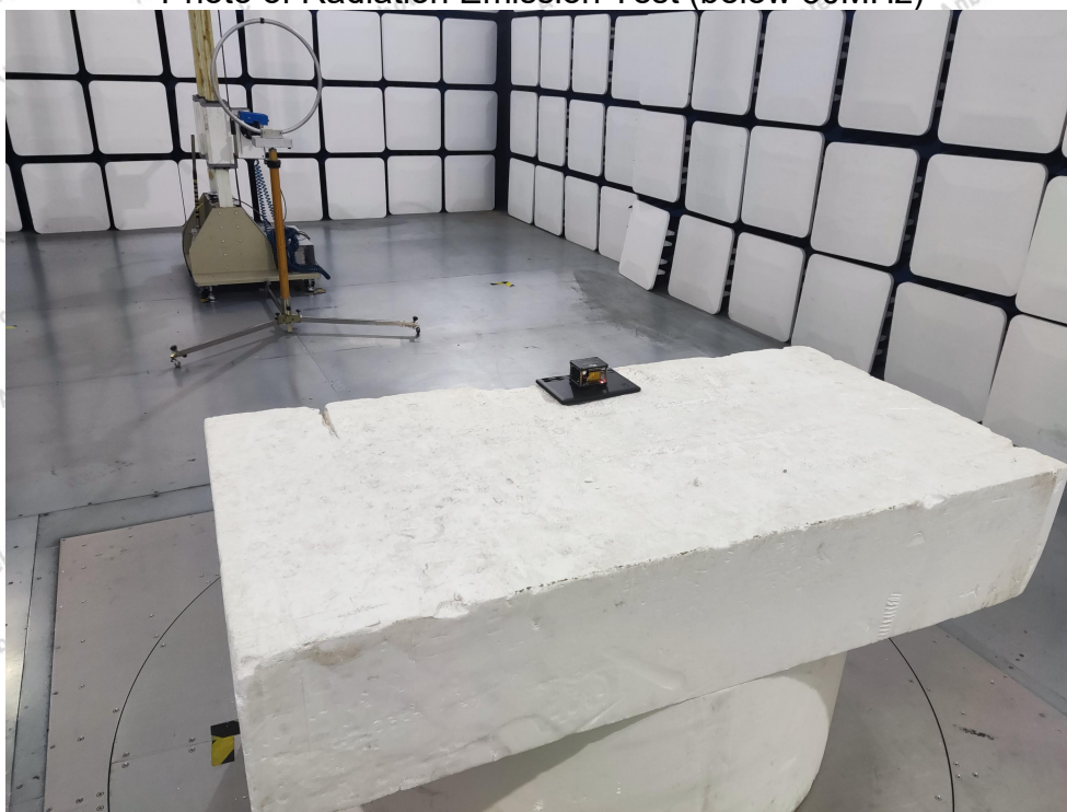
Photo of Radiation Emission Test (below 30MHz)
