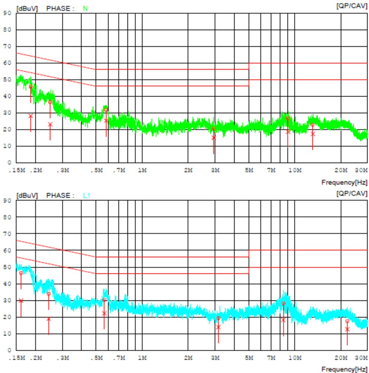
**AC Line Conducted Emissions (List) = TM 1 & Test Channel : Middle****Results of Conducted Emission**
