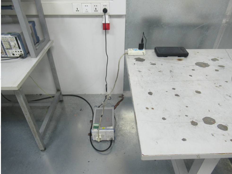
Photo of Conducted Emission Measurement
