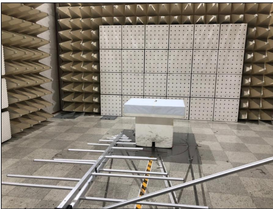
**- Photo of Radiated Spurious Emission Test (Above 1 GHz)**
